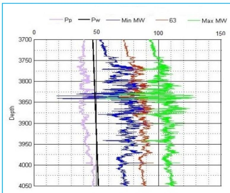
Figure 4- safe and unsafe sections in wellbore wall instability in terms of depth
