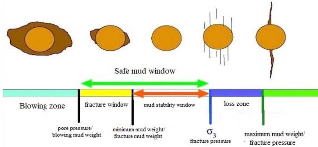
Figure 1- safe and unsafe sections in wellbore wall stability
