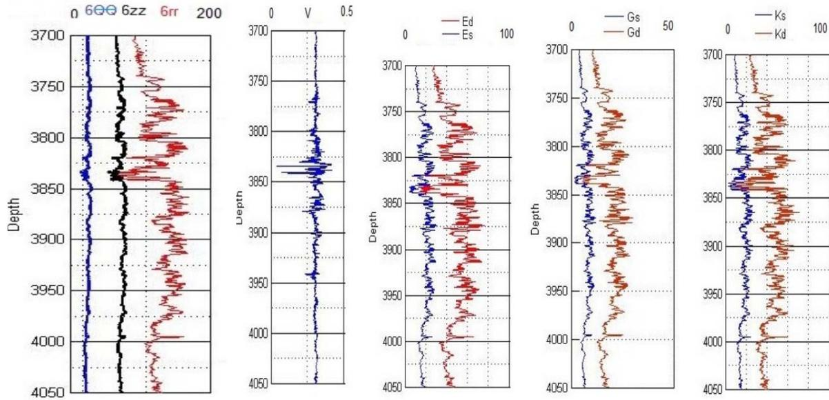
Figure 3- Dynamic and static moduli (four right charts) and axial, tangential and radial induced stresses in depth (left chart)
