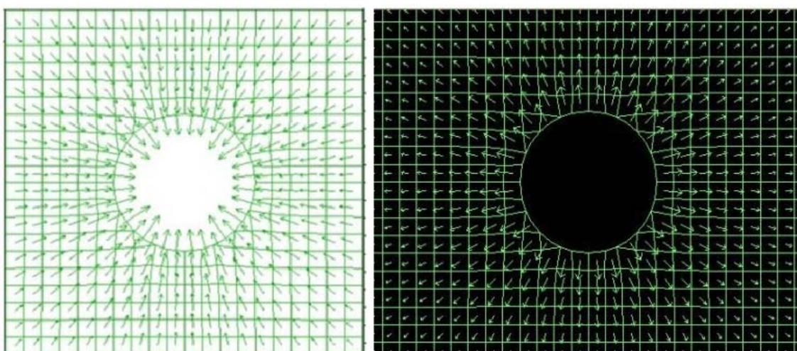
Figure 6- Permeation of mudflow vectors into the formation in over- balanced (right) and Permeation of mudflow vectors into the formation in balanced (left) modes
