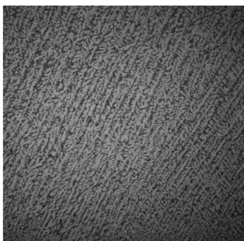
Fig. 5. 1417M alloy casting bottom part structure after MHDO
