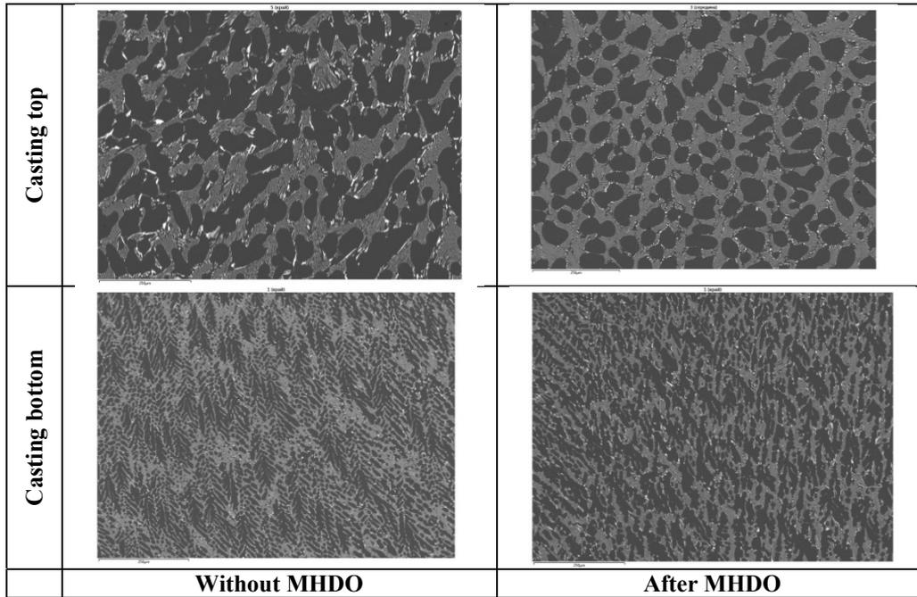
Fig. 3.1417M alloy casting microstructure
