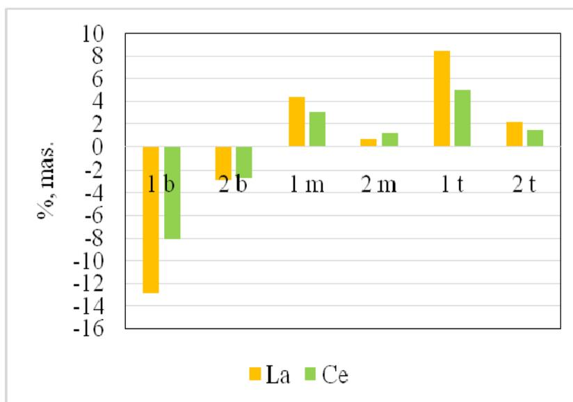
Fig. 2. Results of La and Ce content determination in ingots without MHDO (1) and after MHDO (2) (b – ingot bottom, m – ingot middle, t – ingot top)
