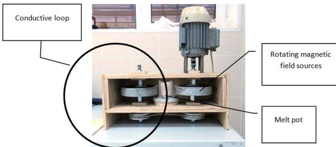
Fig. 1. External view of MHDO unit for molten aluminium alloys
