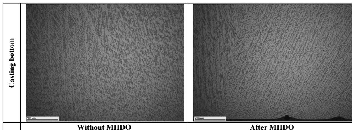
Fig. 4.1417M alloy casting microstructure
