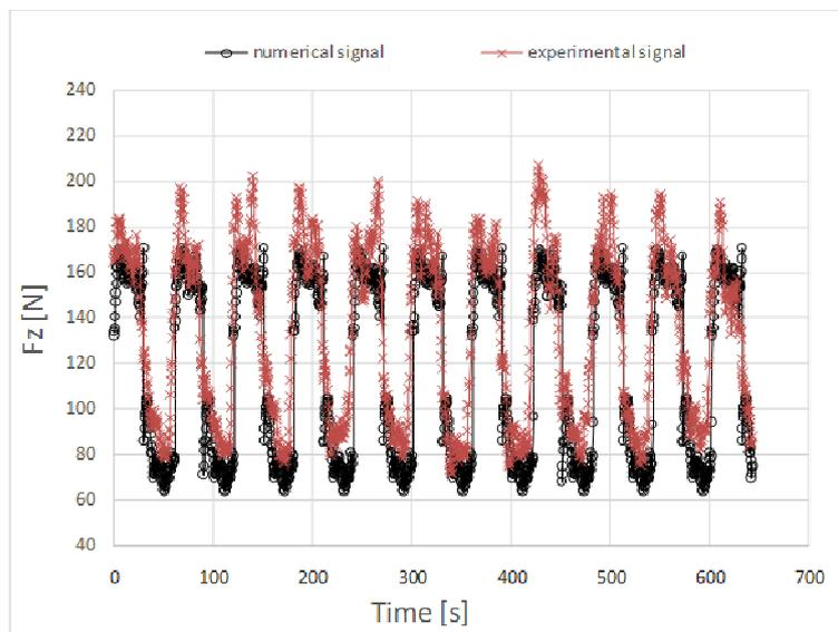
Figure 16. Example of time domain signal monitored in Z direction for a mill with six inserts
