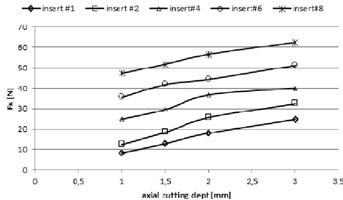
Figure 20. Average  $F_x$  vs.  $P_a$  with the change of the number of inserts: Feed per tooth “ft” 0.022 mm;  $V_t$  100 m/min
