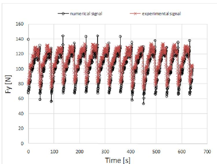
Figure 18. Example of time domain signal monitored in Y direction for a mill with eight inserts
