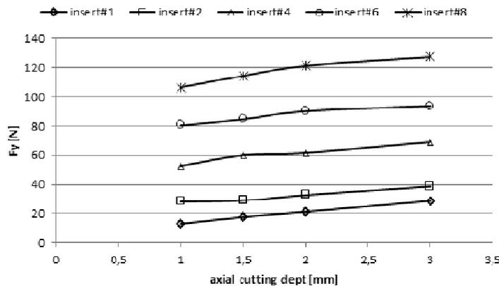
Figure 22. Average  $F_y$  vs.  $P_a$  with the change of the number of inserts: Feed per tooth “ft” 0.022 mm;  $V_t$  100 m/min
