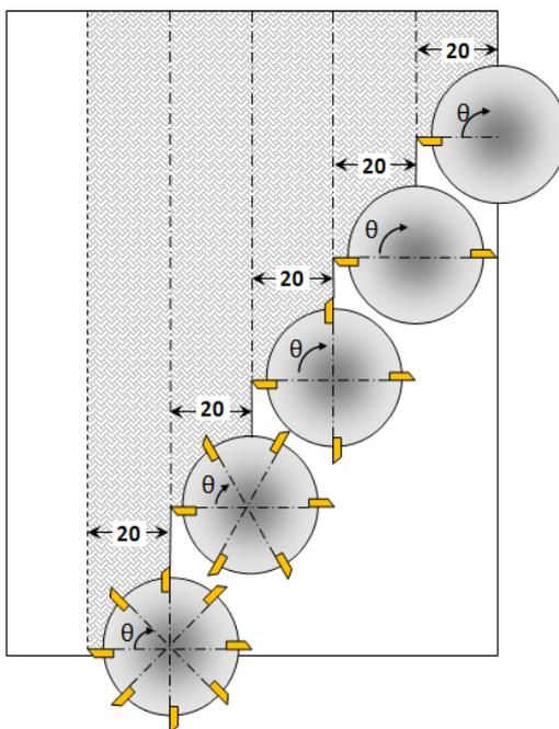
Figure 4. Typologies of mills with 1,2,4,6 and 8 inserts
