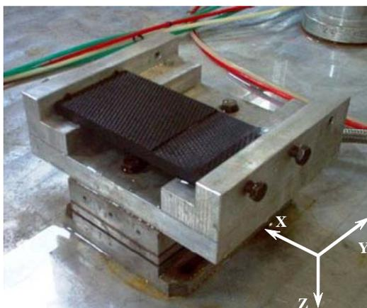
Figure 5. Gripping system/dynamometer/sample
