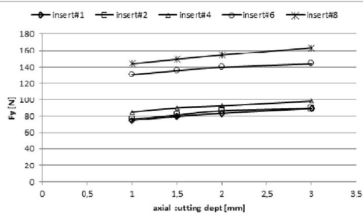
Figure 23. Max Fy vs. Pa with the change of the number of inserts: Feed per tooth “ft” 0.022 mm; Vt 100 m/min
