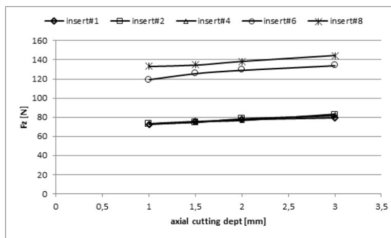
Figure 27. Max Fz vs. Pa with the change of the number of inserts: Feed per tooth “ft” 0.022 mm; Vt 300 m/min
