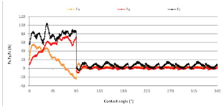
Figure 6. Time domain signal monitored in X, Y and Z direction for one tool revolution
