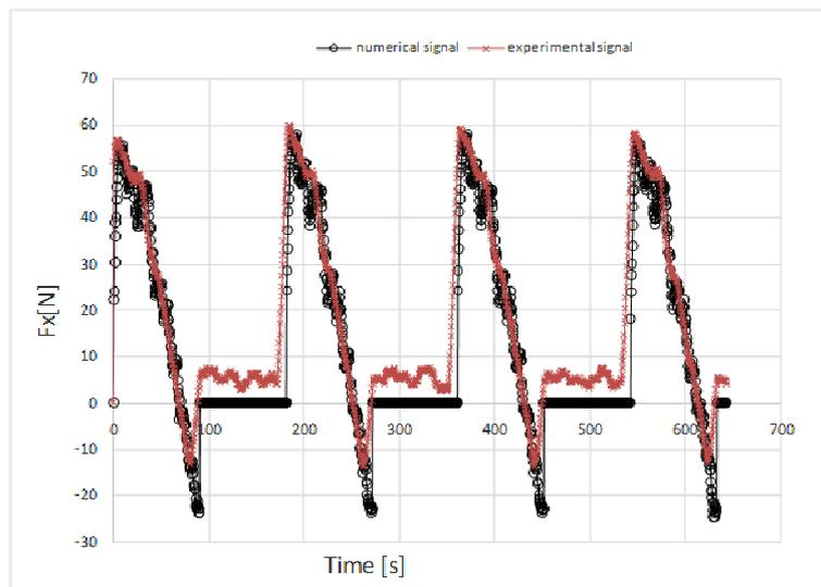
Figure 8. Example of time domain signal monitored in X direction for a mill with two inserts
