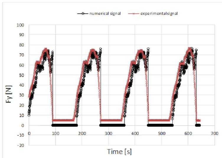
Figure 9. Example of time domain signal monitored in Y direction for a mill with two inserts
