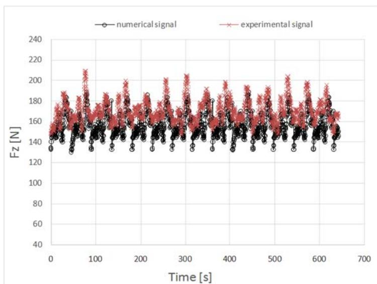
Figure 19. Example of time domain signal monitored in Z direction for a mill with eight inserts
