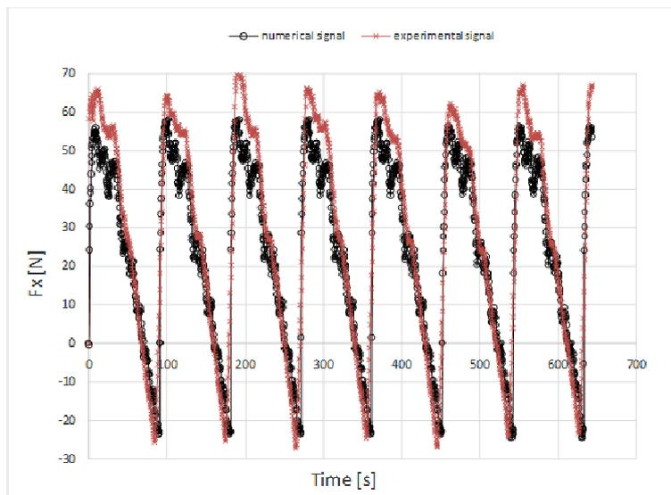
Figure 11. Example of time domain signal monitored in X direction for a mill with four inserts
