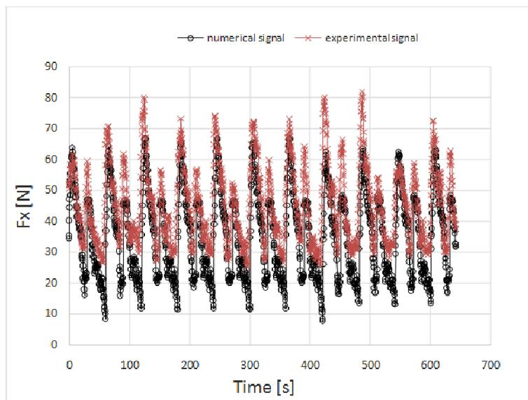
Figure 14. Example of time domain signal monitored in X direction for a mill with six inserts
