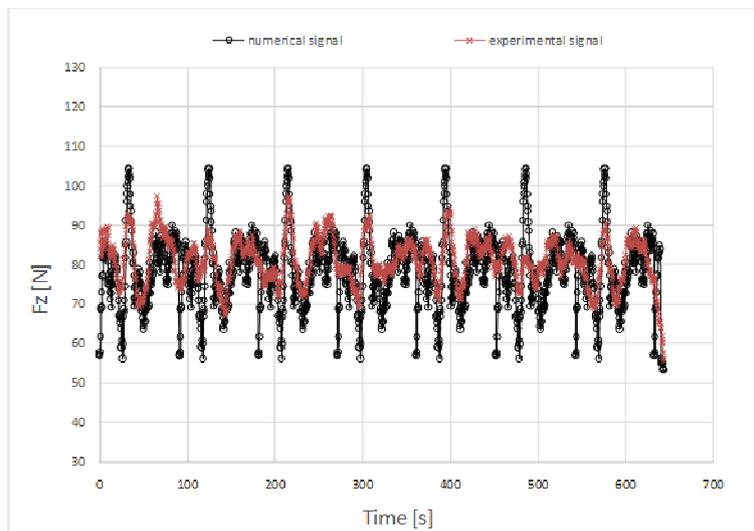
Figure 13. Example of time domain signal monitored in Z direction for a mill with four inserts
