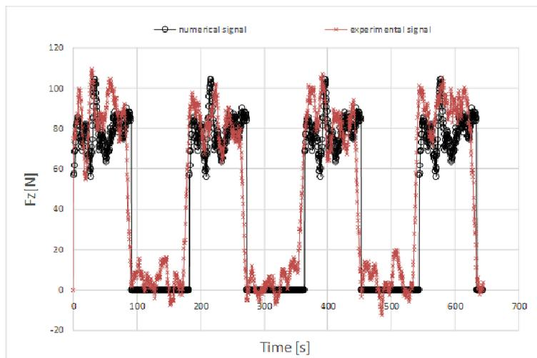
Figure 10. Example of time domain signal monitored in Z direction for a mill with two inserts
