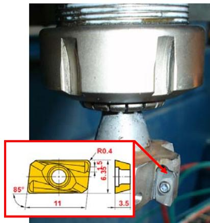
Figure 2. Milling Tool with one insert
