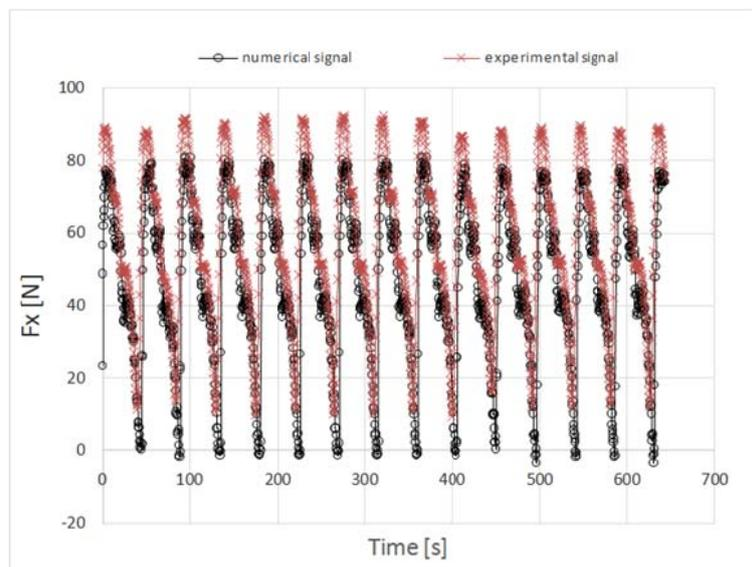
Figure 17. Example of time domain signal monitored in X direction for a mill with eight inserts
