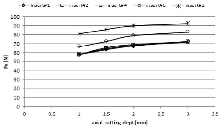
Figure 21. Max  $F_x$  vs.  $P_a$  with the change of the number of inserts: Feed per tooth “ft” 0.022 mm;  $V_t$  100 m/min
