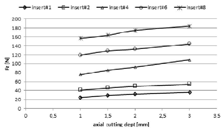
Figure 24. Average Fz vs. Pa with the change of the number of inserts: Feed per tooth “ft” 0.022 mm; Vt 100 m/min
