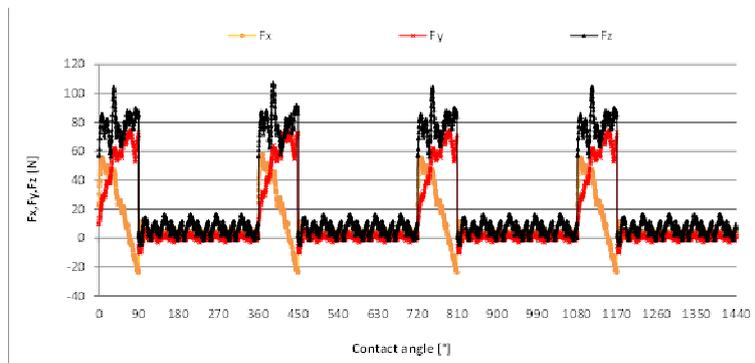
Figure 7. Time domain signal monitored in X, Y and Z direction for four tool revolutions
