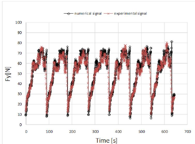
Figure 12. Example of time domain signal monitored in Y direction for a mill with four inserts
