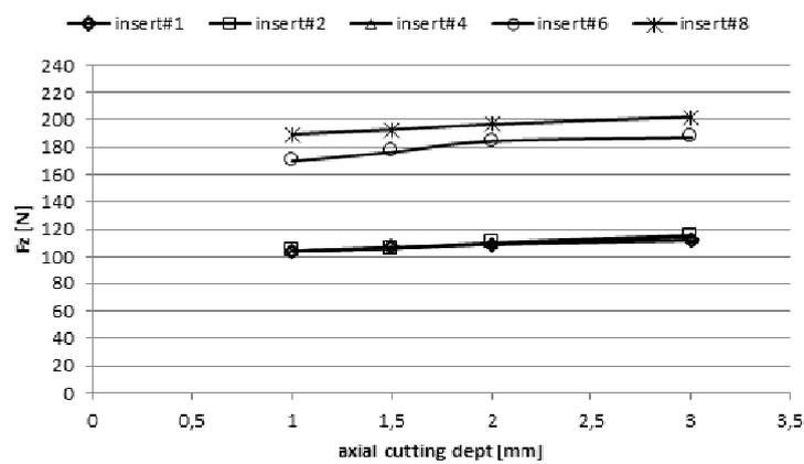
Figure 25. Max Fz vs. Pa with the change of the number of inserts: Feed per tooth “ft” 0.022 mm; Vt 100 m/min
