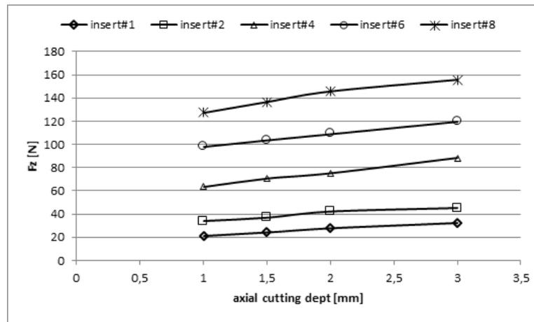
Figure 26. Average Fz vs. Pa with the change of the number of inserts: Feed per tooth “ft” 0.022 mm; Vt 300 m/min
