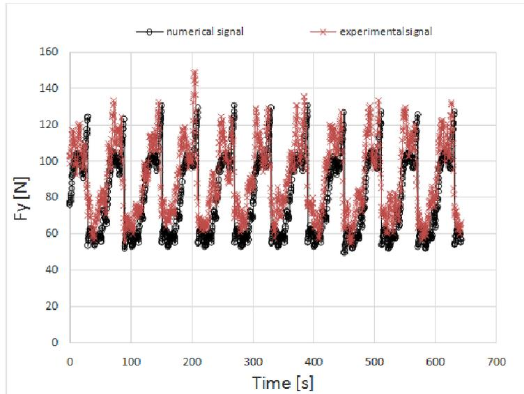
Figure 15. Example of time domain signal monitored in Y direction for a mill with six inserts
