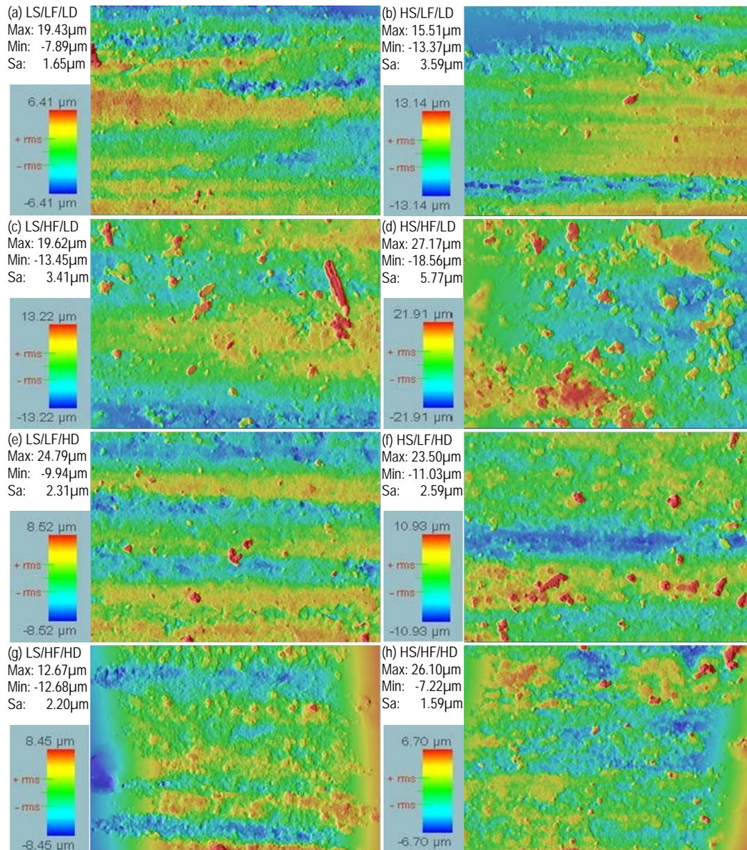
Fig. 5. (a-h) Profilometer images workpiece ground with coolant L-Low; H-High; S-Speed; F-Feed; D-Depth of cut
