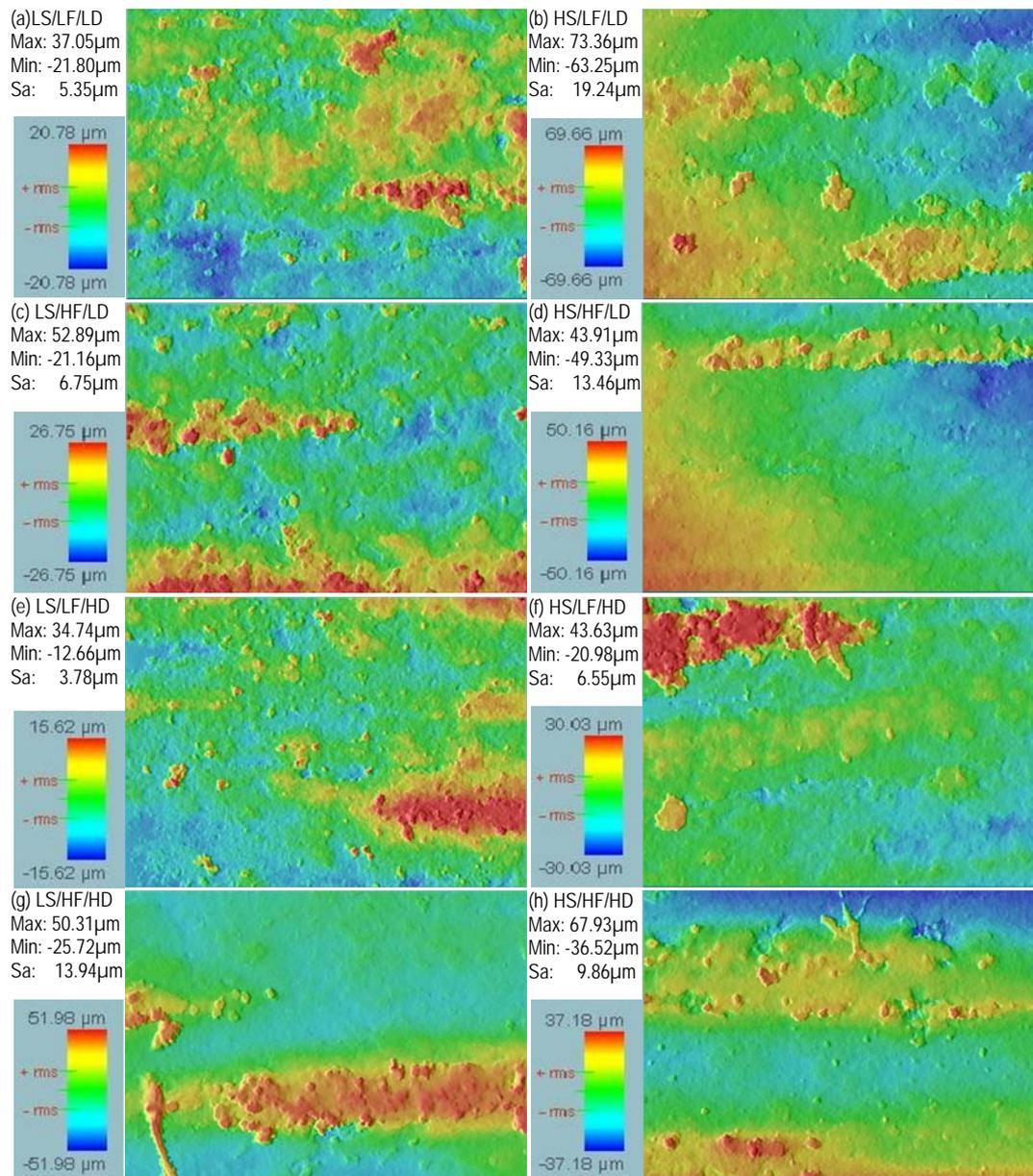
Fig. 4. (a-h) Profilometer images workpiece ground in dry condition L-Low; H-High; S-Speed; F-Feed; D-Depth of cut
