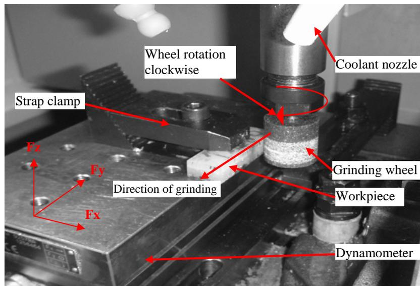
Fig. 1. Grinding experimental setup
