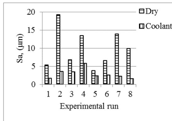
Fig. 3. Surface area roughnesses (Sa) for different experimental runs
