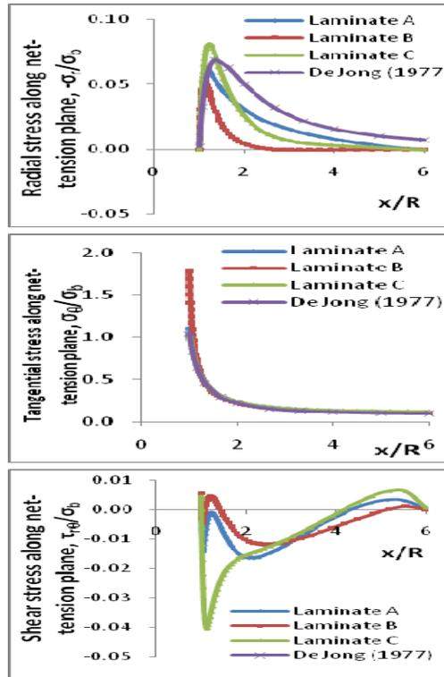
Fig. 3: Effect of laminate properties upon stress distribution along net-tension plane.
