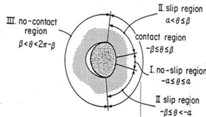
Fig. 5: Contact interaction at pin/hole boundary (after Hyer and Klang, 1987)
