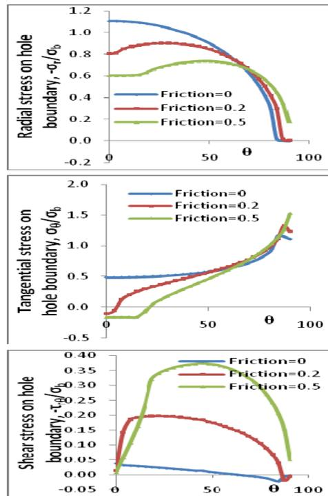
Fig. 6: Effect of friction upon stress distribution of Laminate A on hole boundary
