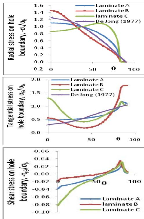
Fig. 4: Effect of laminate properties upon stress distribution on hole boundary.
