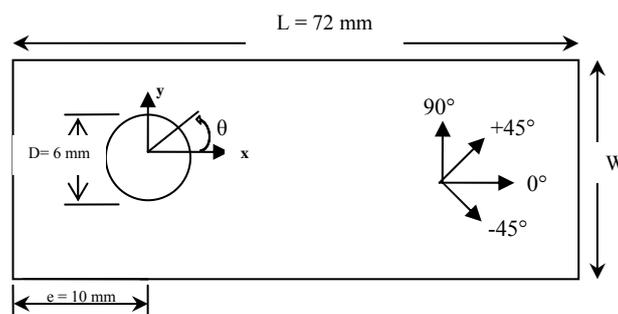
Fig. 2: Geometry of the composite laminate specimens
