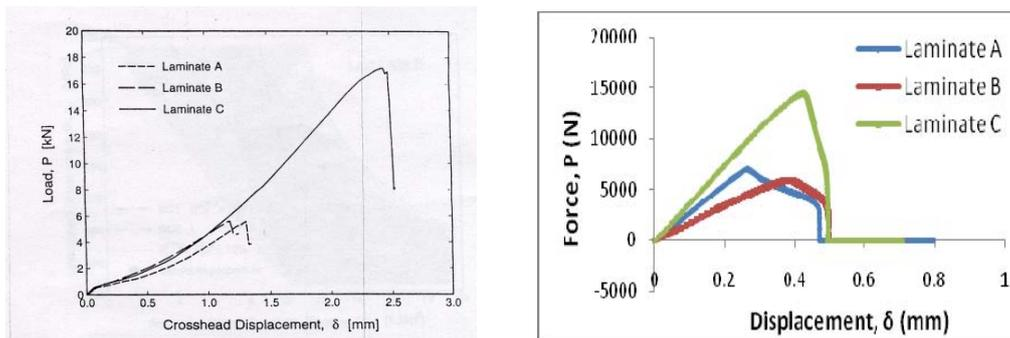
Fig. 8: Comparison of experimental work (left, Hollmann (1986)) and full contact CZM model (right).
