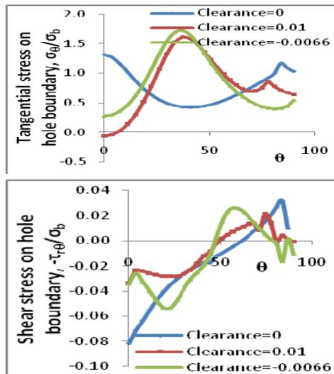
Fig. 7: Effect of clearance upon stress distribution of Laminate C on hole boundary
