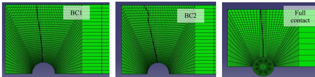
Fig. 10: Crack propagation of XFEM results with effects of boundary conditions.
