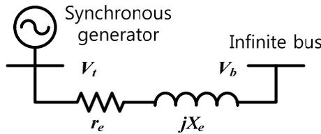
Fig. 5. Single-machine infinite bus system
