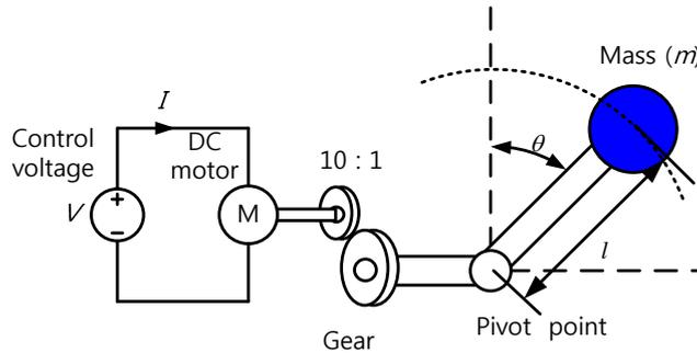
Fig. 2. Inverted pendulum controlled by a DC motor
