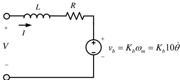
Fig. 3. Model of an armature-controlled DC motor
