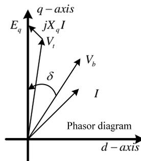
Fig. 6. Steady state phasor diagram of the SMIB system
