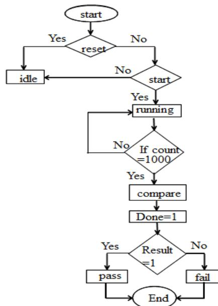
Fig.12 Flowchart representing the implementation of the signals used
