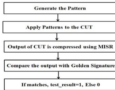
Fig.11 Design Flow representation of the testing process
