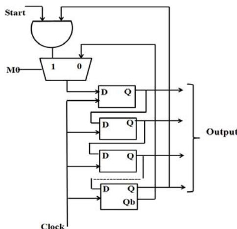
Fig.10 Reconfigurable Twisted Ring Counter
