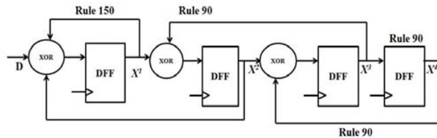
Fig.7. 4-bit HCA using rule 90 and 150
