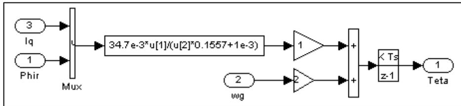
Figure 6. The Rotor field angle generation block
