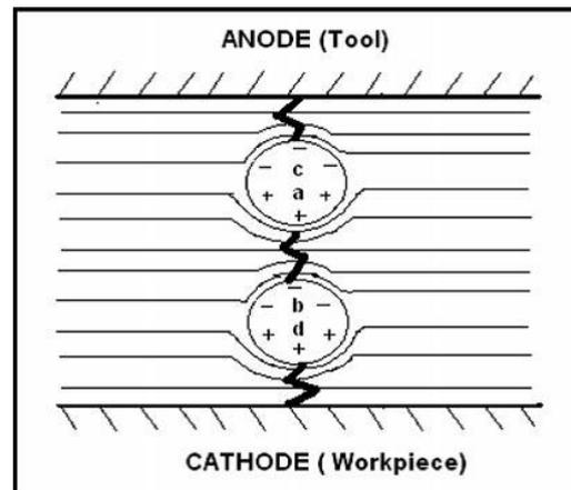
Fig.1. Schematic representation of series of discharge in PMEDM [16,18].
