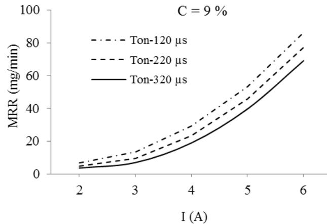
Fig. 4. I and  $T_{ON}$  vs. MRR
