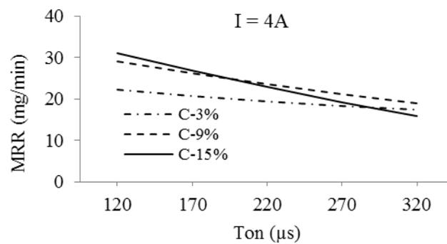
Fig. 5.  $T_{ON}$  and C vs. MRR
