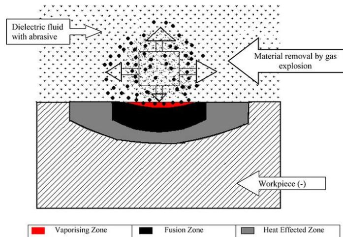
Fig. 2. Material removal by gas explosion during PMEDM [16, 17]
