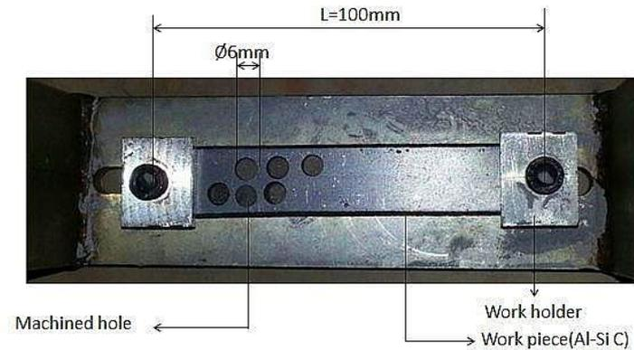
Fig. 3(a). Clamped work piece showing dimensions
