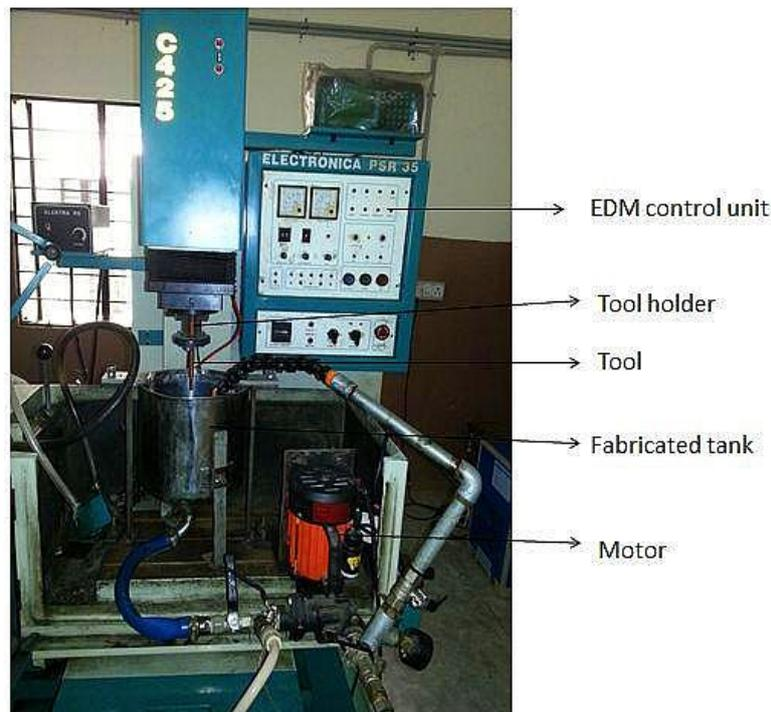
Fig. 3(b). Photograph of experimental setup
