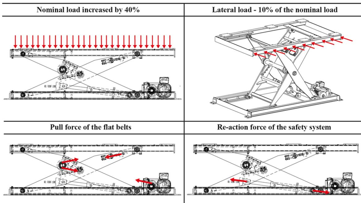
Fig. 8. Loads applied to the scissor lifting table in the structural analysis
