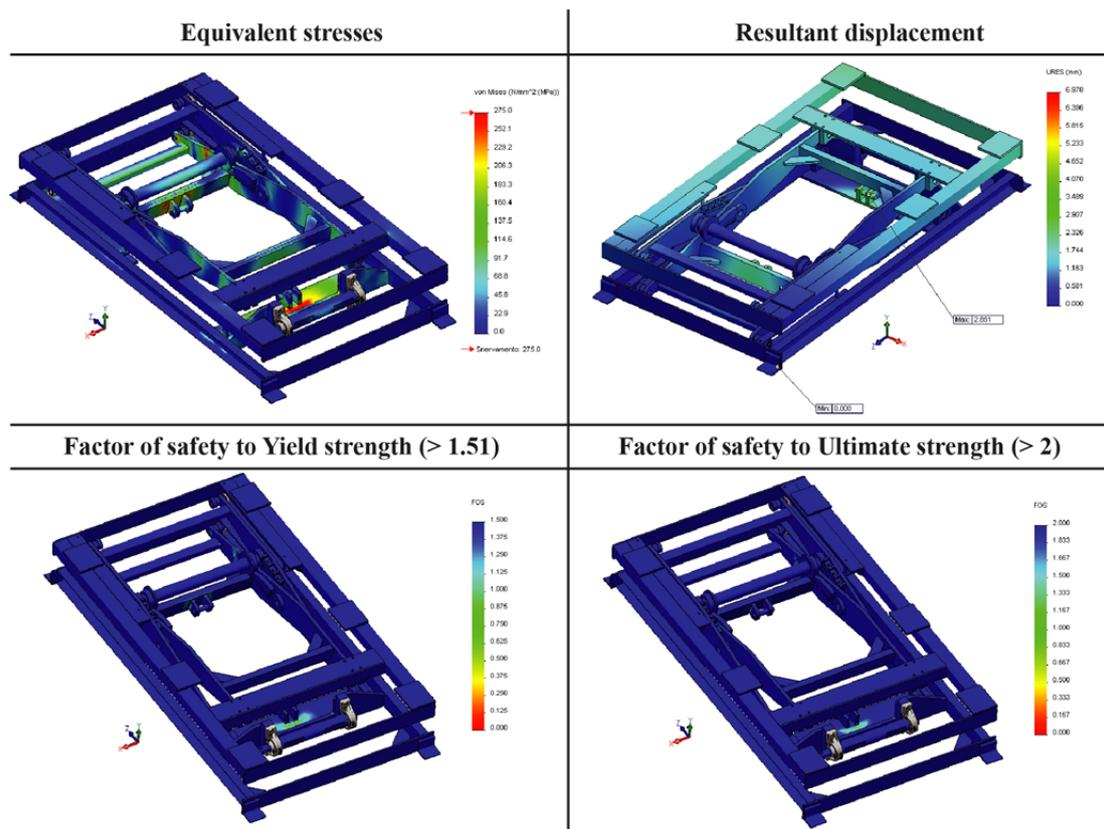
Fig. 10. Results of structural analysis for the close lifting table
