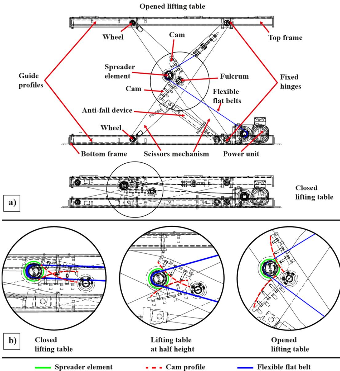
Fig. 11. a) The belt drive scissor lifting table, b) The scissor mechanism movements of the new table
