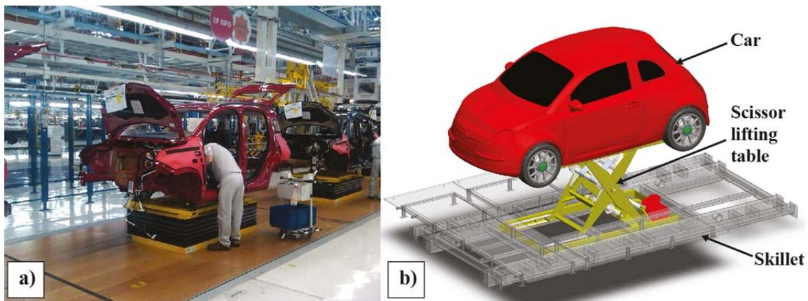
Fig. 2. Handling line: a) Men at work; b) CAD model of the scissor lifting table
