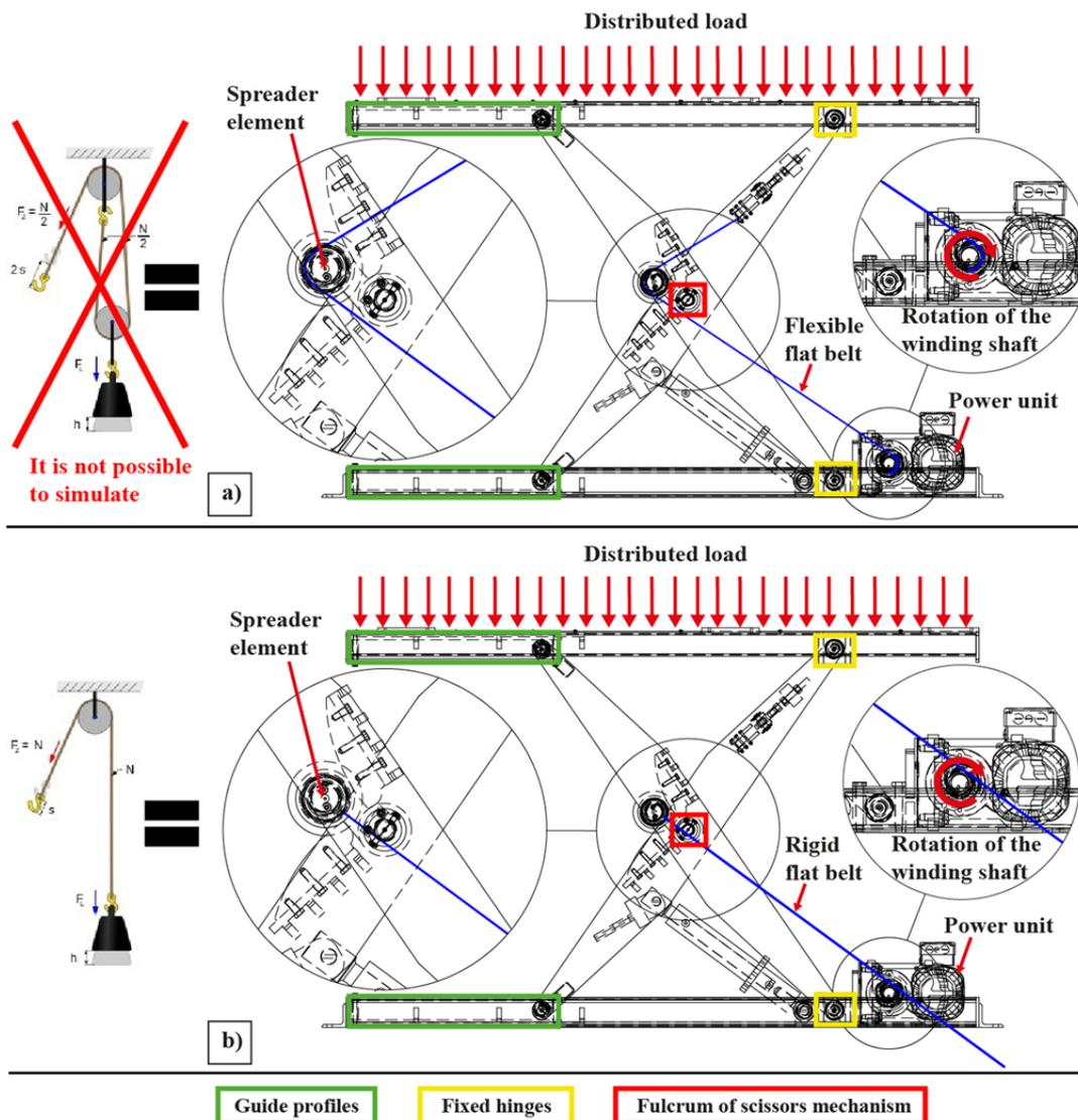
Fig. 5. Scissor lifting table: a) the design case, b) the simulated case
