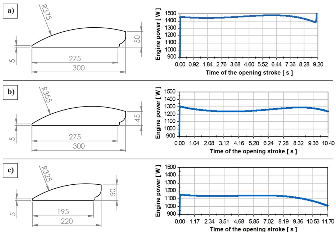
Fig. 6. Results of the iterative approach to design the cam profile
