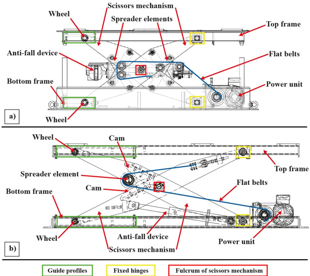
Fig. 3. Scissor lifting tables: a) commercial lifting table, b) new lifting table
