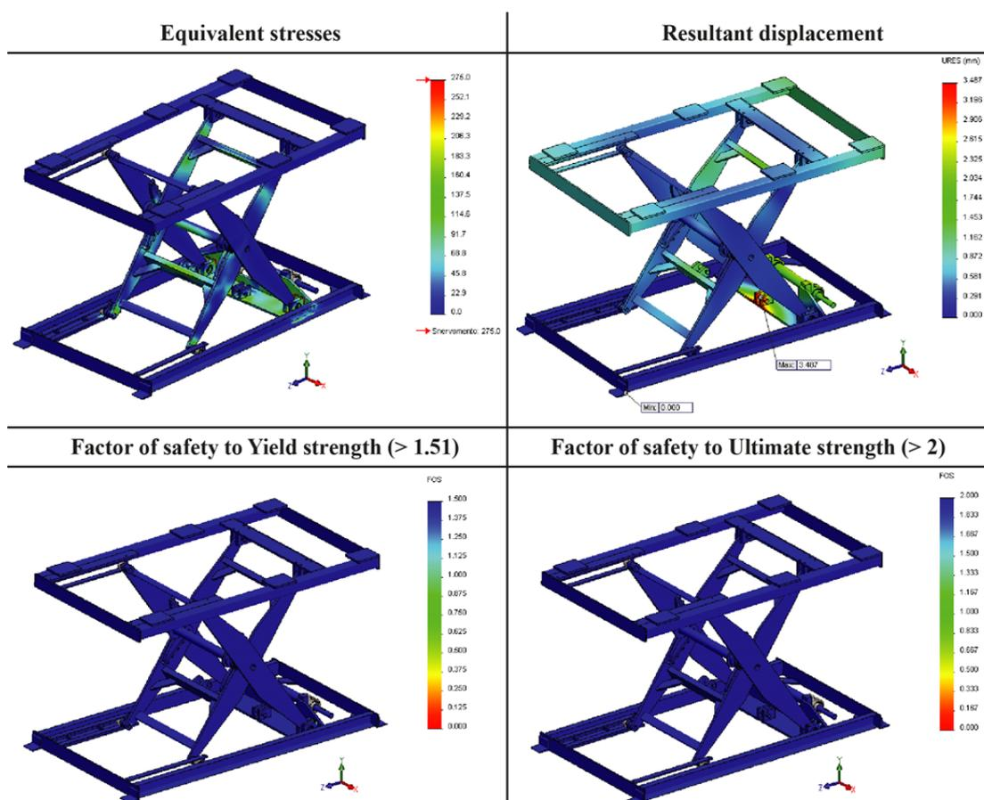
Fig. 9. Results of structural analysis for the open lifting table
