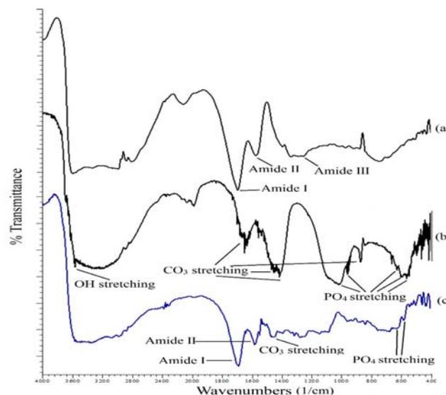
Fig. 3 FTIR spectra of (a) FGel, (b) FHAp, and (c) non-irradiated FHAp/FGel composite
