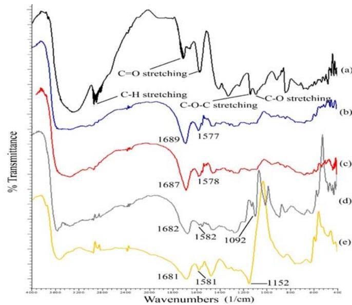
Fig. 4 FTIR spectra of non-irradiated of (a) PVA, and FHAp/FGel-PVA composite at FGel/PVA percent mass ratio of (b) 10/0, (c) 7.5/2.5, (d) 5.0/5.0, and (e) 2.5/7.5 (w/w)
