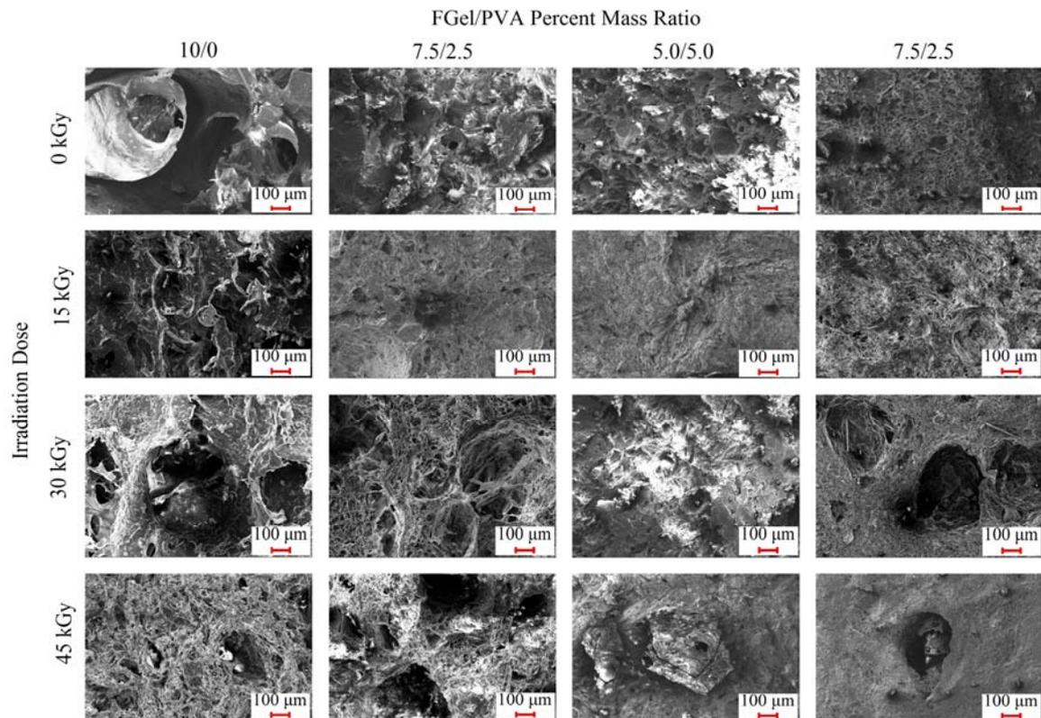
Fig. 7 SEM micrograph of pores of irradiated FHAp/FGel based composite at varied FGel/PVA percent mass ratio and irradiation doses
