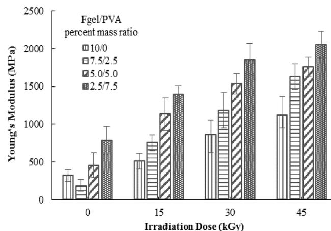
Fig. 2 Young's modulus ( $E$ ) of irradiated FHAp/FGel based composite at varied FGel/PVA mass ratio
