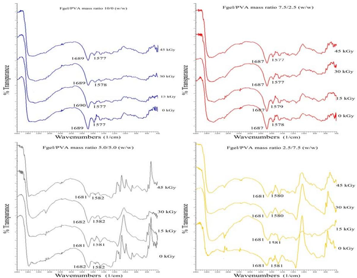
Fig. 5 FTIR spectra of irradiated FHAp/FGel based composite at varied FGel/PVA percent mass ratio
