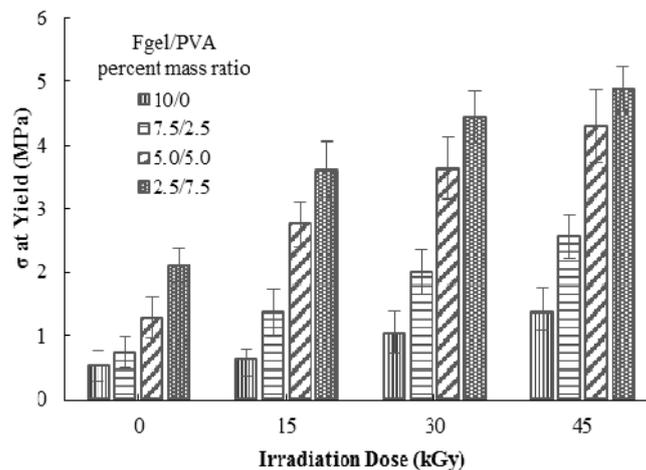
Fig. 1 Compressive strength at yield ( $\sigma$ ) of irradiated FHAp/FGel based composite at varied FGel/PVA mass ratio
