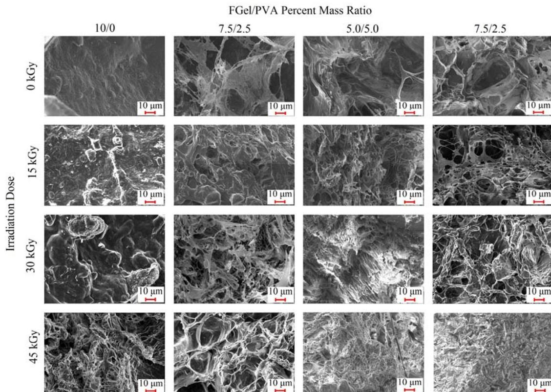
Fig. 6 SEM micrograph of surface roughness of irradiated FHAp/FGel based composite at varied FGel/PVA percent mass ratio and irradiation doses
