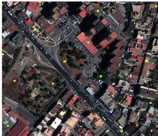
Figure 7: Training sites of shadowed (red) and free shadow (yellow) zones on the pan-sharpened RGB composition.
