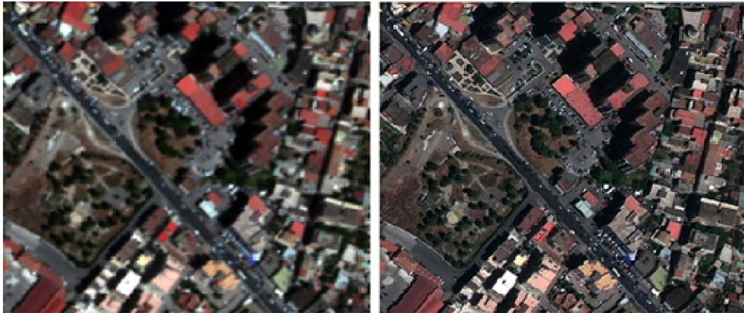
Figure 2: Comparison between RGB composition of multispectral (left) and pan-sharpened (right) band.
