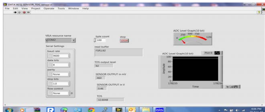
Fig. 10 LabVIEW Front Panel showing TDS values
