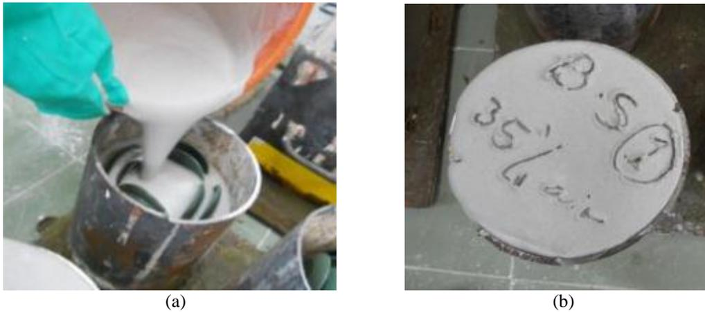
Fig. 2. Molding process where, (a) slurry with excellent flowability could be poured easily into the metal flask and (b) harden slurry forming a block mold.
