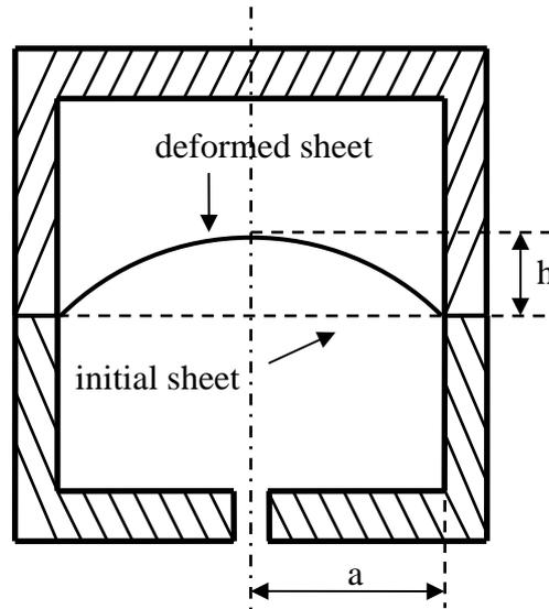
Fig. 1. Example of free forming process: the draw shows the deformed metal sheet
