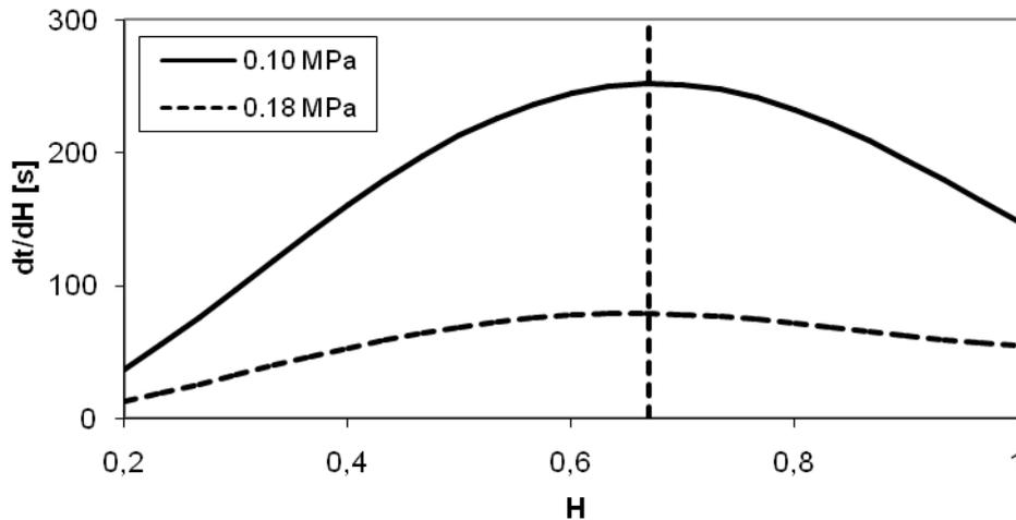
Fig. 7. PbSn60 alloy: experimental tests results in terms of  $(dt/dH)$ -H curve; the  $H^*$ -value is equal to 0.67 at a temperature of 298K and at pressures of 0.10 and 0.18 MPa
