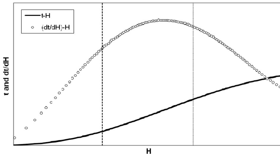
Fig. 2.  $t$ - $H$  and  $(dt/dH)$ - $H$  curves for a constant pressure in the free forming process of a circular sheet
