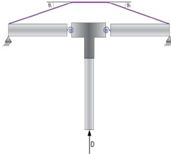
Fig. 2. T-joint Nonlinear FE Model (1-inch and 2-inch)
