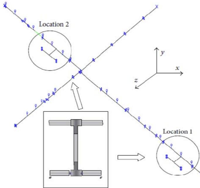
Fig. 5. Main Piping System with two nonlinear T-joint Systems
