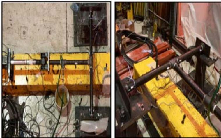
Fig. 1. T-joint Test Setup, Conducted by University at Buffalo [10-11]
