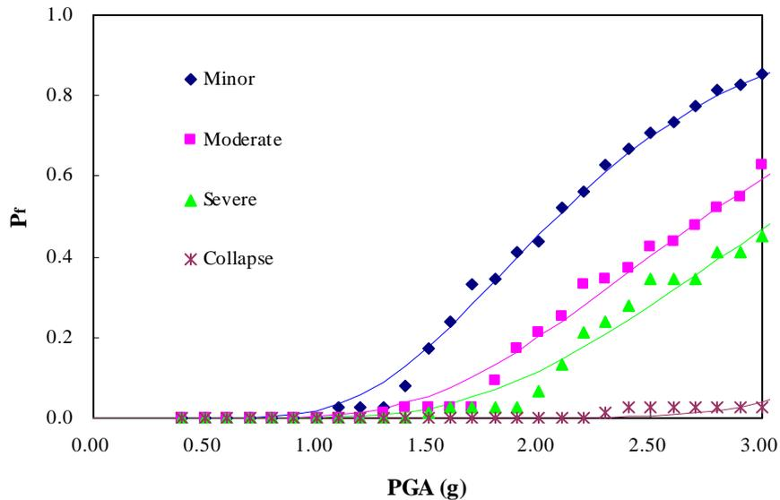
Fig. 8. Piping Fragility of 1-inch Threaded T-joint at Location 2
