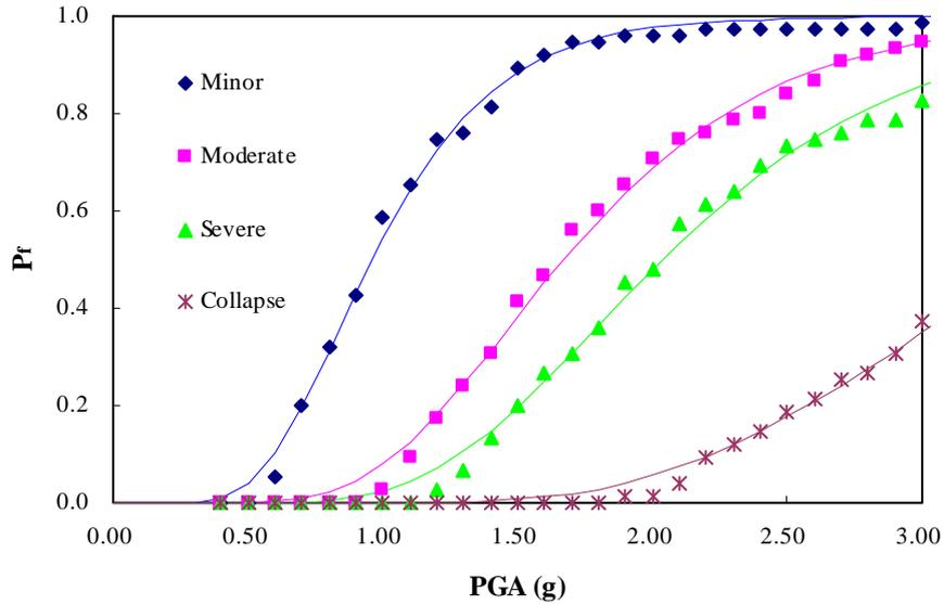
Fig. 7. Limit States Corresponding to Ductility Levels
