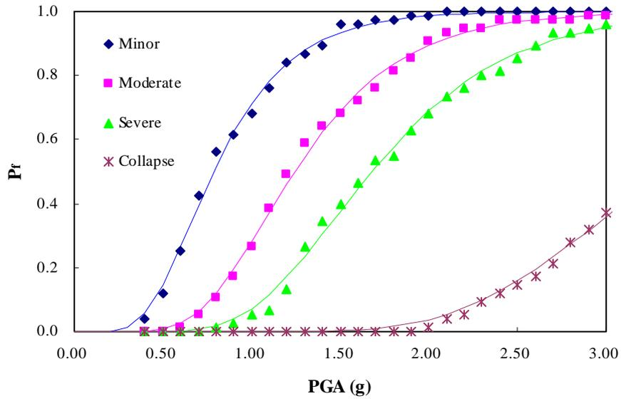
Fig. 9. Piping Fragility of 2-inch Threaded T-joint at Location 1
