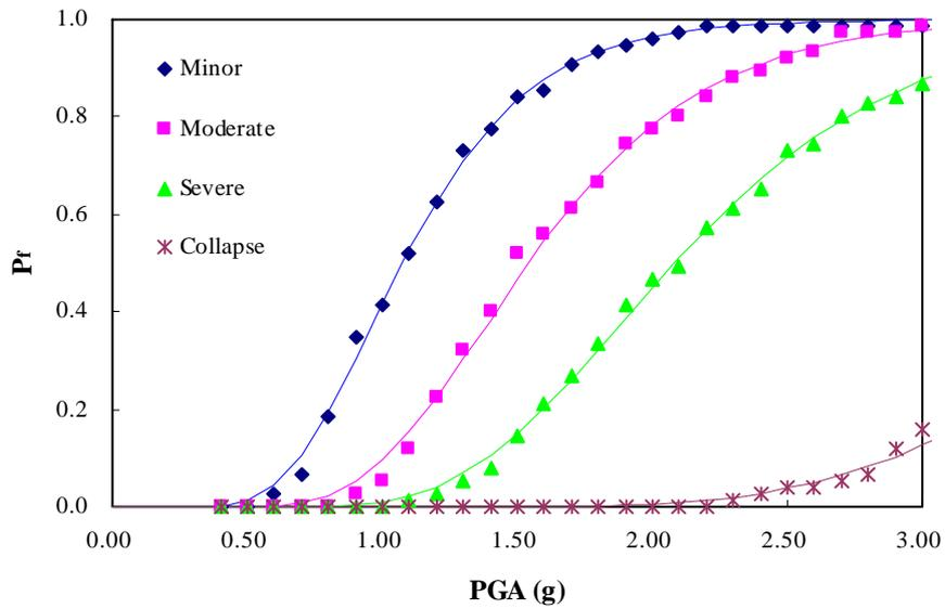
Fig. 10. Piping Fragility of 2-inch Threaded T-joint at Location 2
