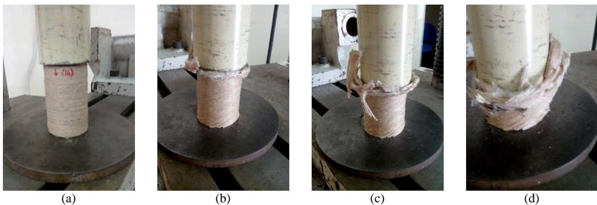
Fig. 6. Progressive collapse of steel/kenaf hybrid tube with [30/-30].
