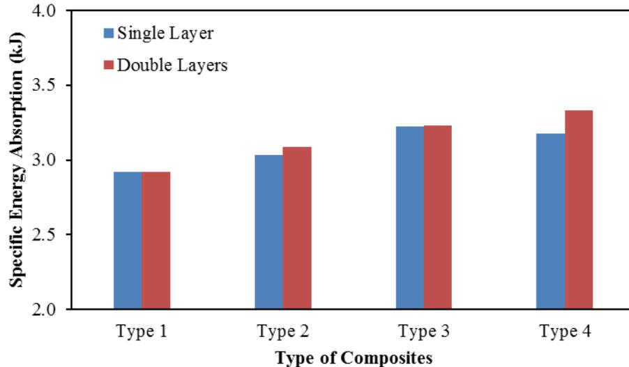
Fig. 5. Effect of hybridizations of steel/kenaf fibre tubes on energy absorption performances for two types of layers.
