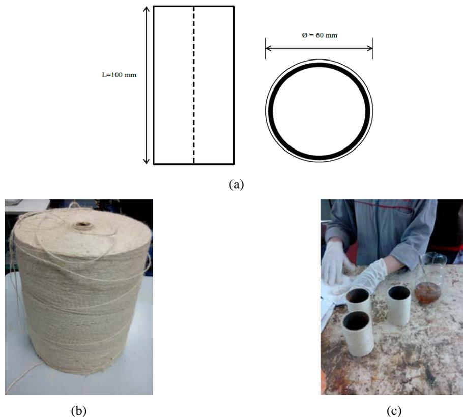
Fig. 1 (a) Kenaf yarn bundle in the as-received condition, (b) The schematic diagram of the steel tube and (c) Completed hybrid kenaf/steel tube composites
