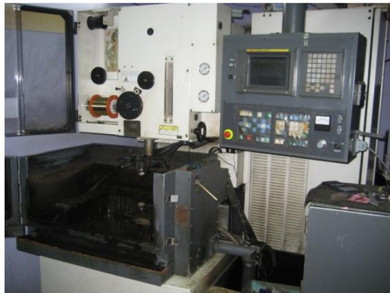
Fig. 1. EDM wire cutting machine
