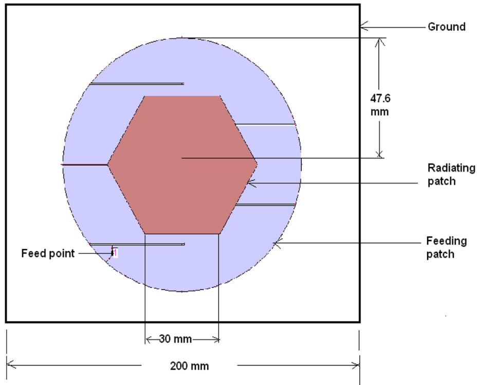
Fig. 2. The geometry of hexagonal radiating patch on circular meander feeding patch
