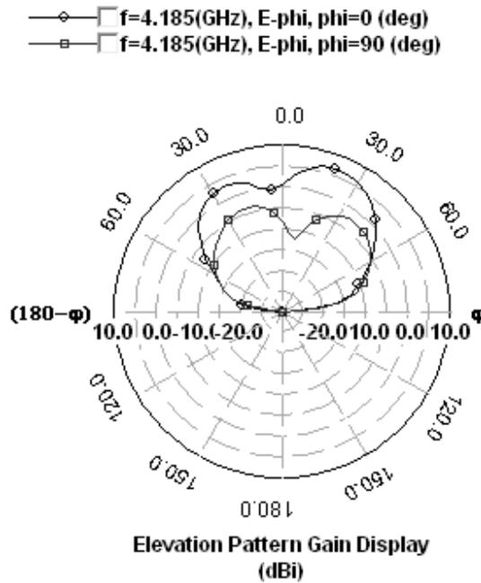
Fig. 16. Elevation Radiation Pattern at 4.185 GHz
