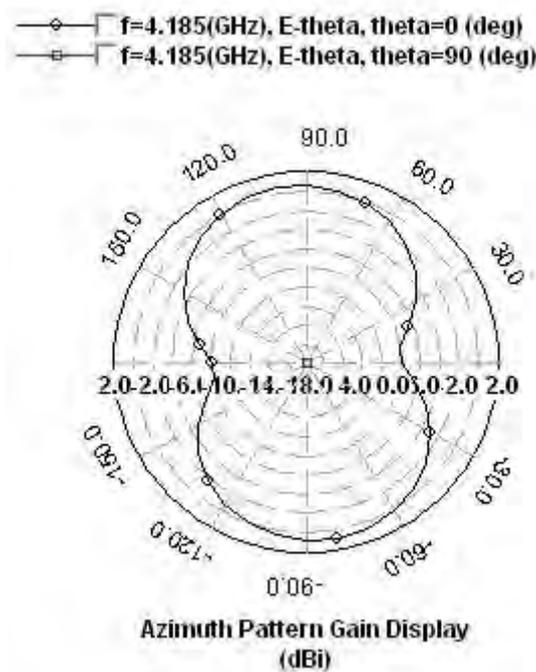
Fig. 17. Azimuthal Radiation Pattern at 4.185 GHz
