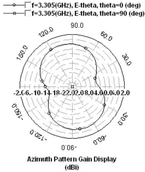
Fig. 15. Azimuth Radiation Pattern at 3.30 GHz
