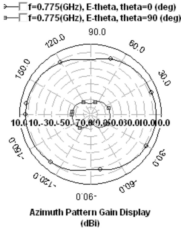
Fig. 13. Azimuthal Radiation Pattern at 0.775 GHz
