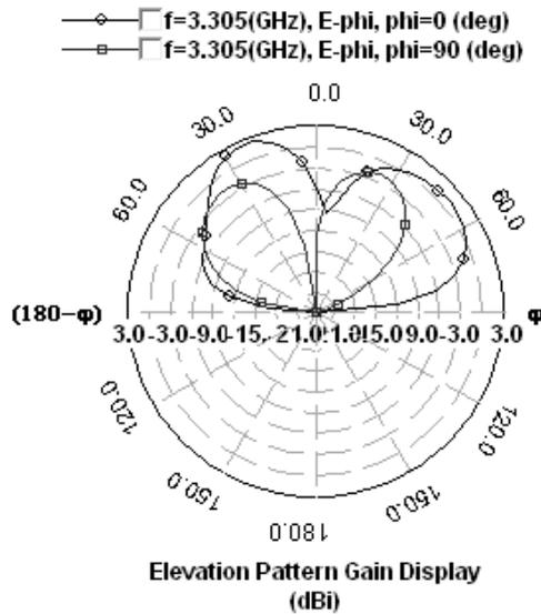
Fig. 14. Elevation Radiation Pattern at 3.30 GHz
