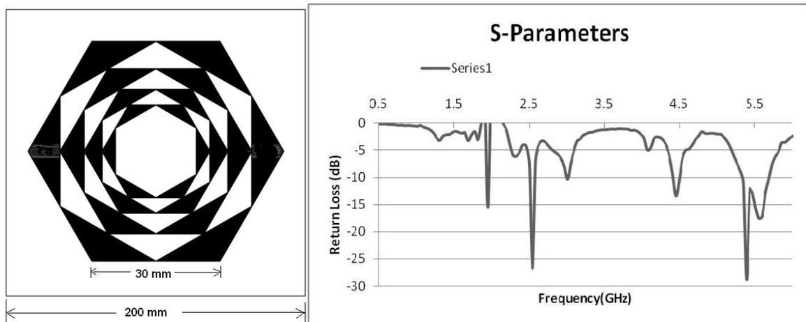
Fig. 3. Hexagonal Fractal Patch and its S-Parameter
