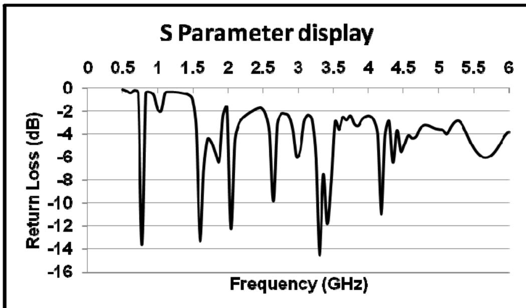
Fig. 7. The Reflection Coefficient Curve Simulation Result of Proposed Fractal Stacked Antenna
