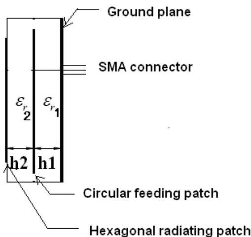
Fig. 1. Stacked structure of the patch antenna side view
