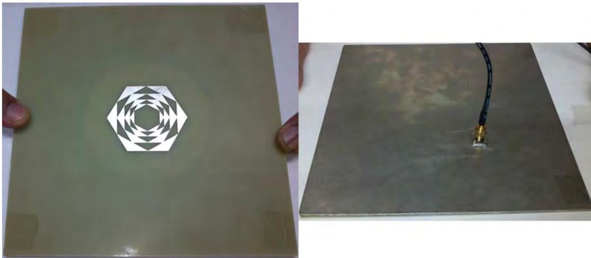
Figure 5. Radiating Upper layer and Lower Ground layer of fabricated antenna
