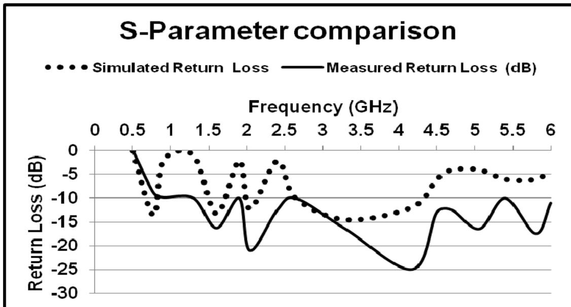
Fig. 11. Comparison of Simulated and Measured Return Loss of Proposed Fractal Stacked Antenna.
