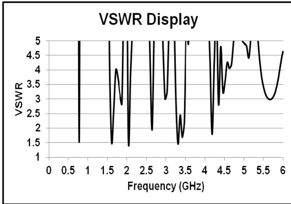
Fig. 8. VSWR Display of the Proposed Antenna
