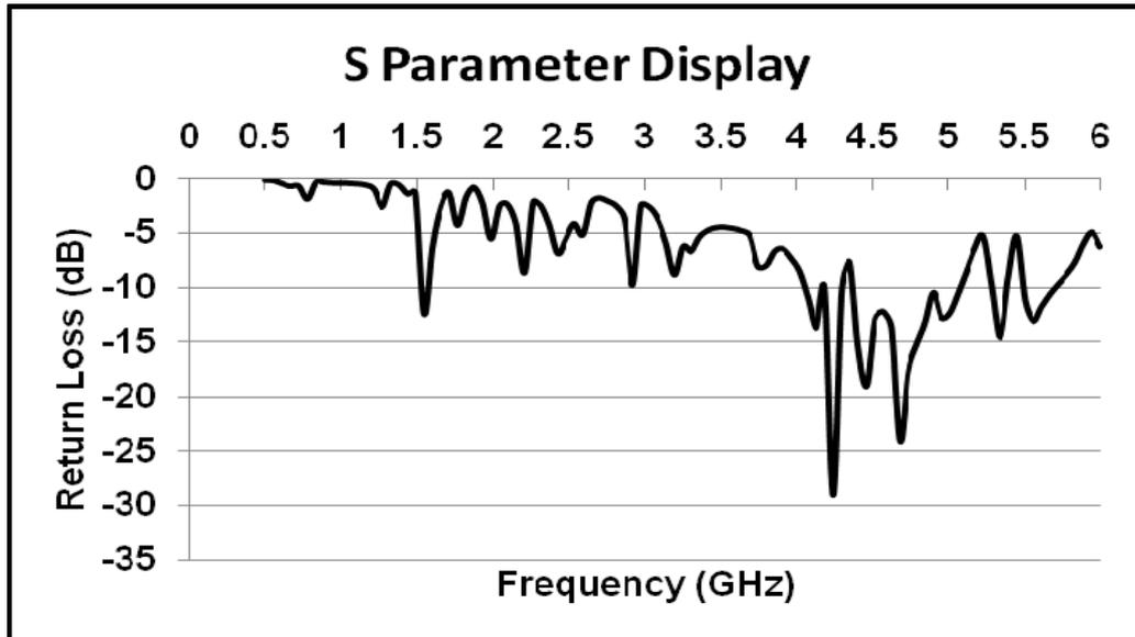
Fig. 6. The reflection coefficient curve of plain hexagonal radiating patch on circular meander patch antenna
