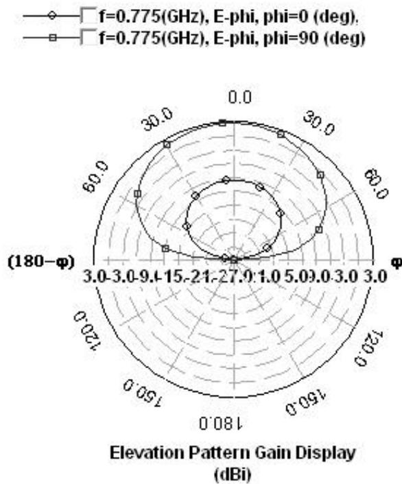
Fig. 12. Elevation Radiation Pattern at 0.775 GHz
