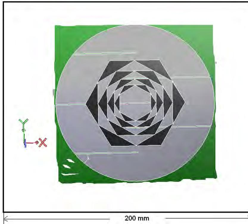
Fig. 4. Proposed Fractal Antenna
