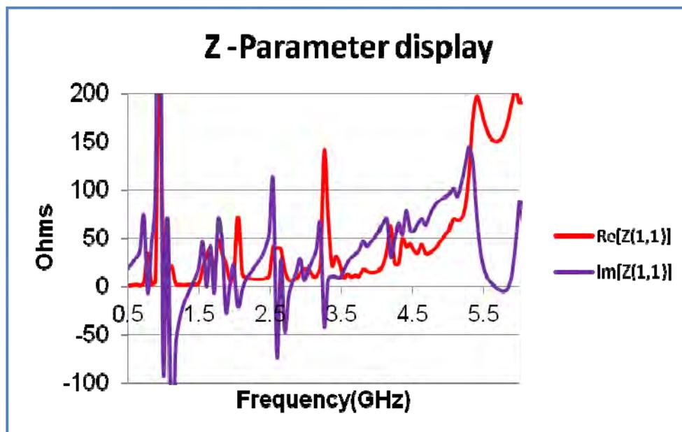
Fig. 9. Z-Parameter of the Proposed Antenna
