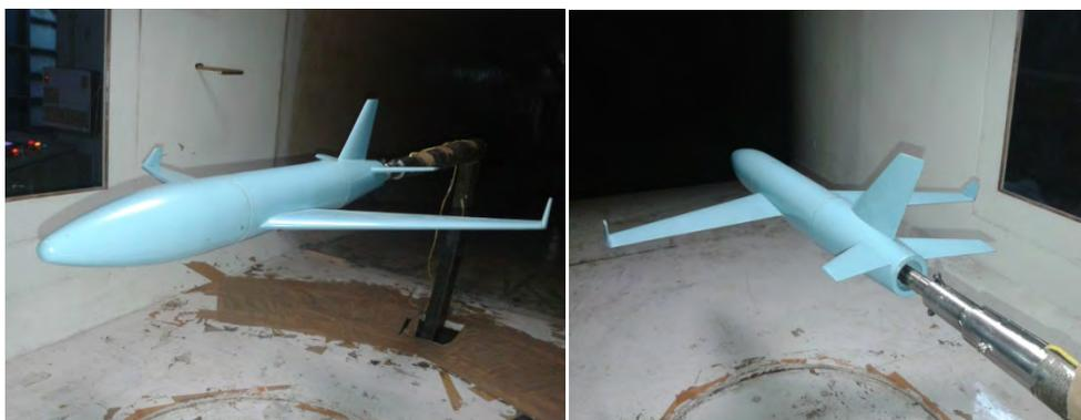
Fig 2. Aircraft model with winglet mounted in the wind tunnel test section
