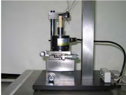
Fig. 2 Assembled X-Y-Z stage to adjust the position of the punch on a specimen
