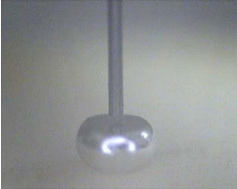
Fig. 4 Pan-cake-shaped solder ball with a diameter of about 800  $\mu\text{m}$  after up-setting and a punch with a diameter of 150  $\mu\text{m}$ .
