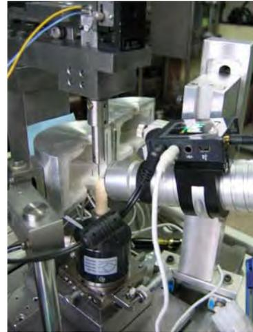
Fig. 3 The assembled impression creep machine
