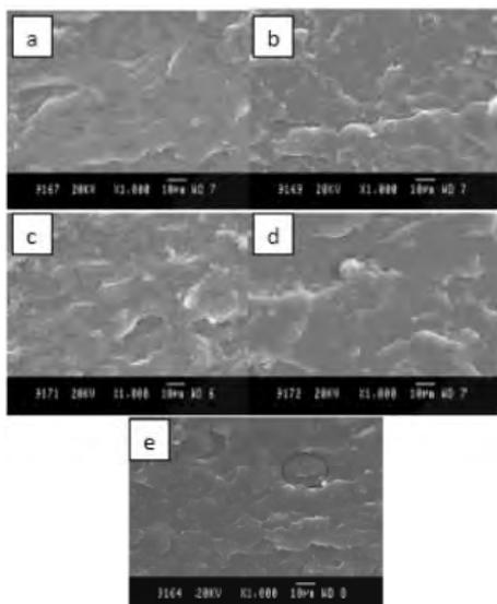
Fig.6. SEM micrograph of hybrid nanocomposites a)PPHNC-1,b)PPHNC-3,c)PPHNC-5, d)PPHNC-7 and e)pure PP
