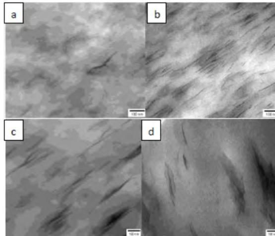
Fig.5. TEM micrograph of hybrid nanocomposites a)PPHNC-1,b)PPHNC-3,c)PPHNC-5 and d)PPHNC-7
