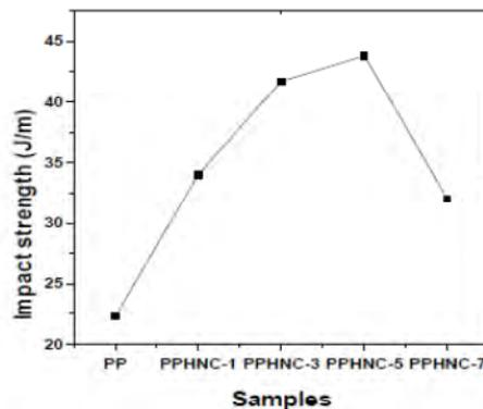
Fig.3.Impact properties of PP and hybrid nanocomposites
