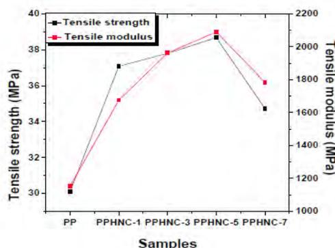
Fig.1. Tensile properties of PP and hybrid nanocomposites
