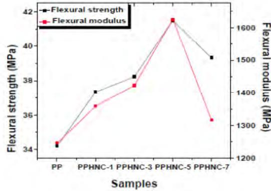
Fig.2.Flexural properties of PP and hybrid nanocomposites
