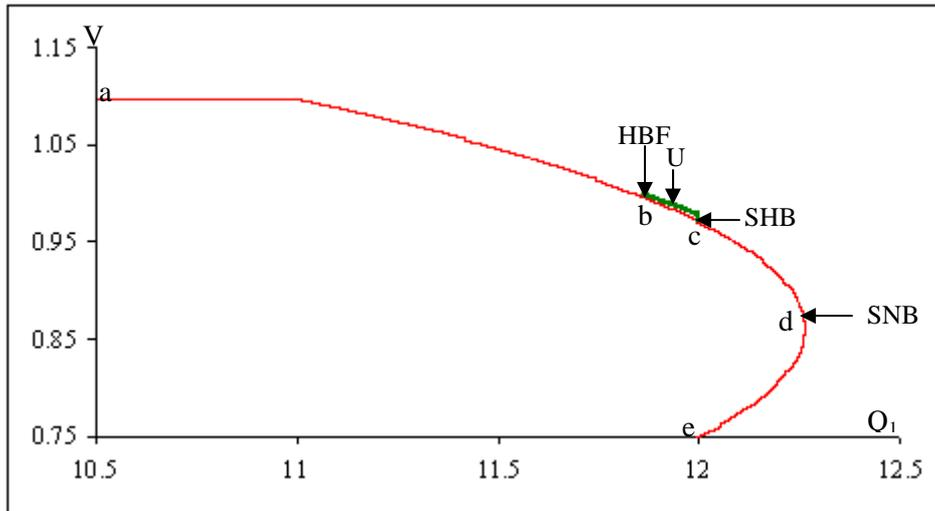
Fig. 10. Bifurcation diagram with SFLC based SVC
