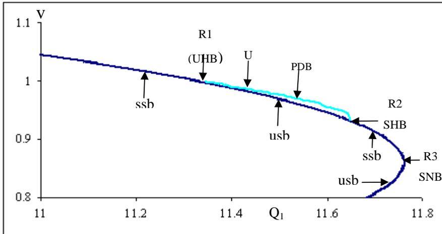
Fig. 6. Bifurcation diagram of load voltage magnitude with conventional SVC
