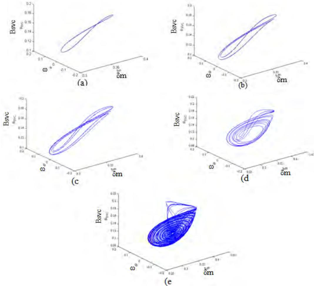
Fig. 8. Cascade of period doubling with conventional SVCe
