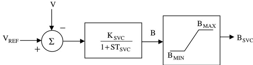
Fig.2 Block diagram representation of Static VAR compensator
