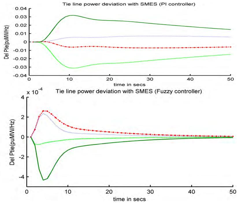
Fig8: Tie line Power deviation of PI and fuzzy controlled four area hydro thermal system with 1% step disturbance at all areas including SMES.
