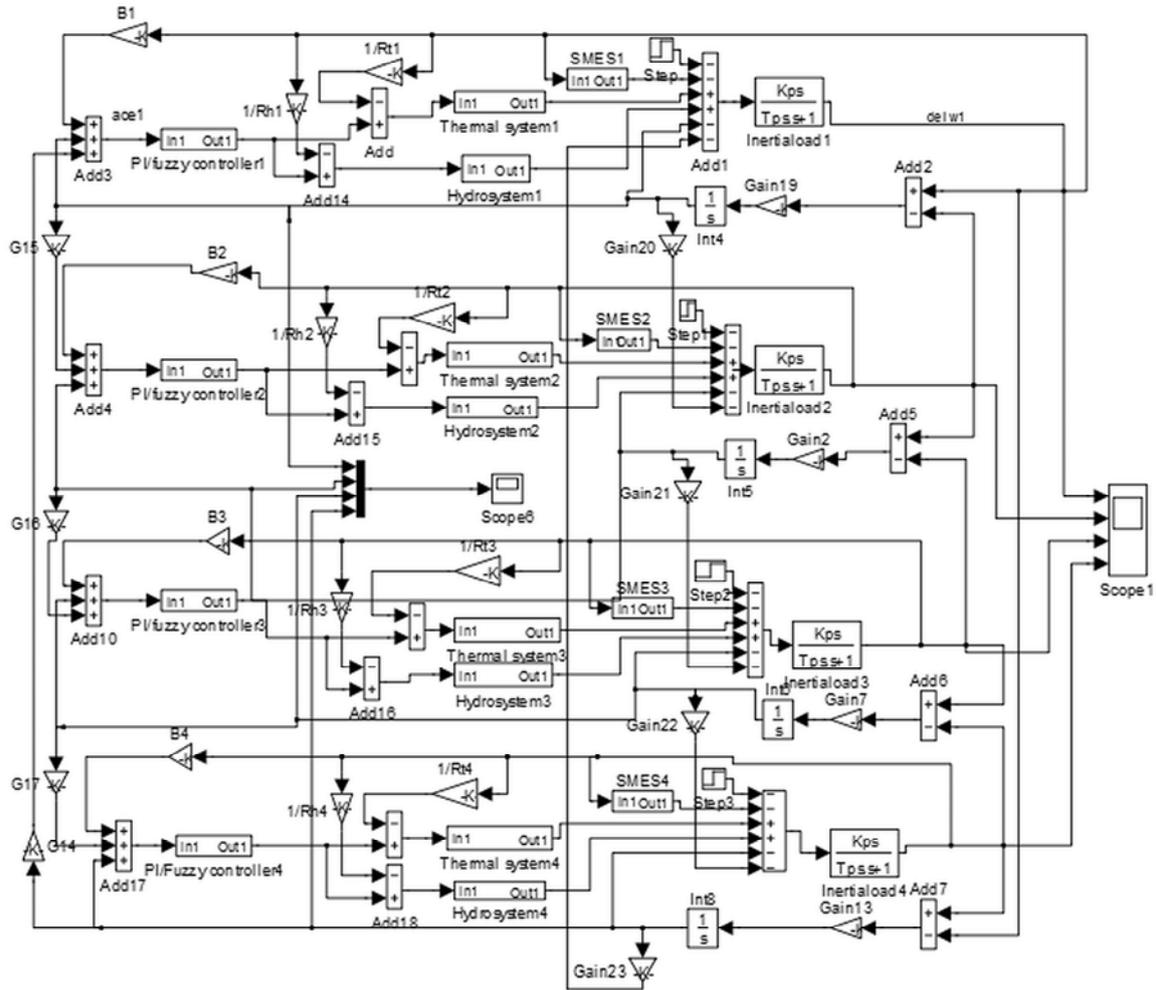
Fig.4. Simulink model for four area hydro thermal system.
