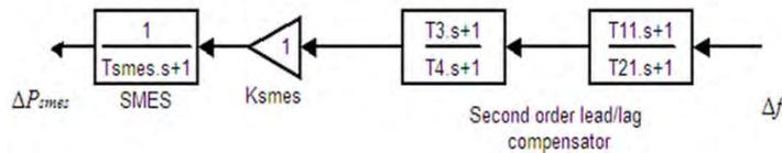
Fig.3. Structure of SMES as frequency stabilizer.
