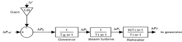
Fig.1. Model of thermal power plant.
