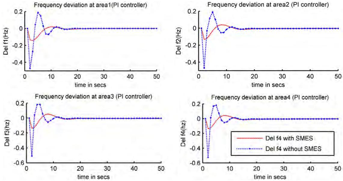
Fig6: Frequency deviation of PI controlled four area hydro thermal system with 1% step disturbance at all areas.
