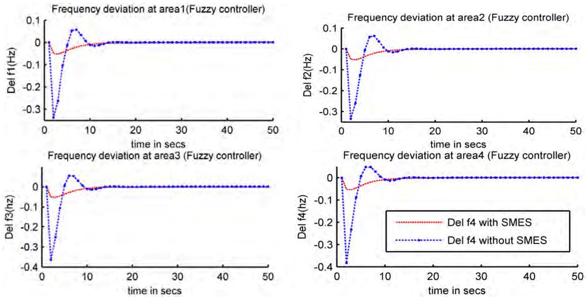
Fig7: Frequency deviation of fuzzy controlled four area hydro thermal system with 1% step disturbance at all areas.
