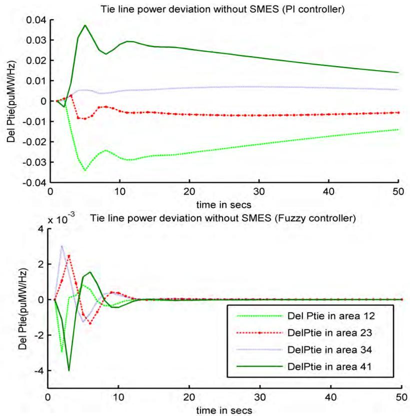
Fig9: Tie line Power deviation of PI and fuzzy controlled four area hydro thermal system with 1% step disturbance at all areas without including SMES.
