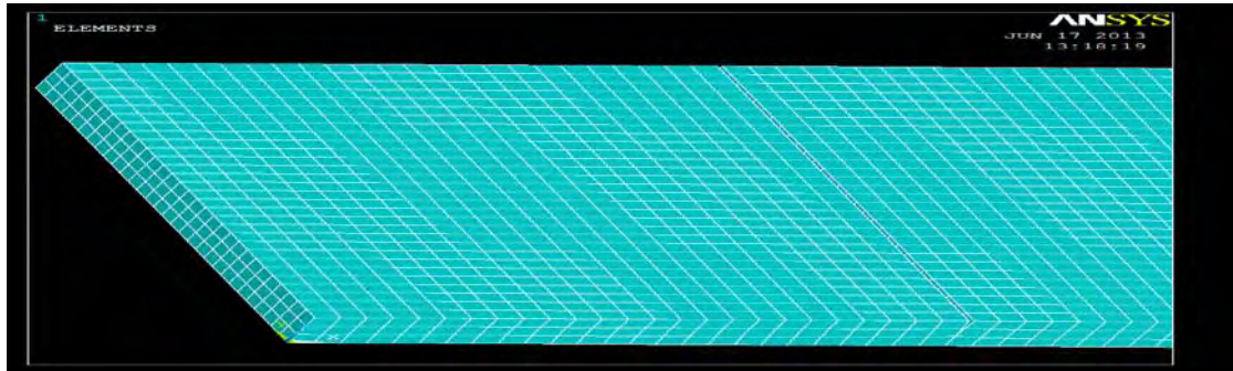
Figure 5: Epoxy E-glass fibre composite cracked beam meshing
