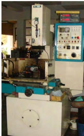
Fig 3. Die sinking microEDM Machining Setup
