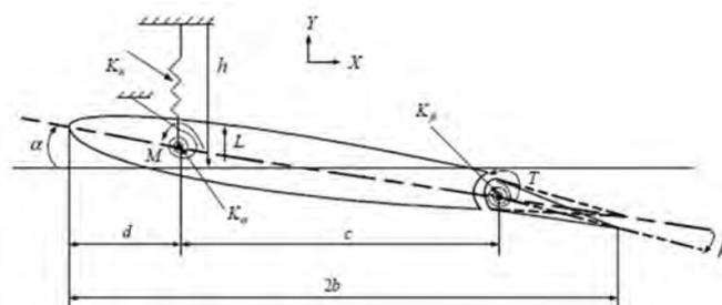
Fig 1. The 2-D wing- flap section of a typical airfoil
