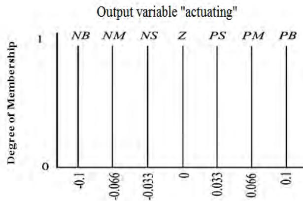
Fig. 5. Defuzzification output voltage variable
