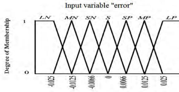
Fig. 3. Fuzzification input voltage variable 1
