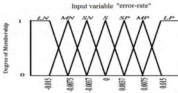
Fig. 4. Fuzzification input voltage variable 2
