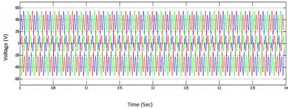
Fig. 7. Voltage waveform without UPQC
