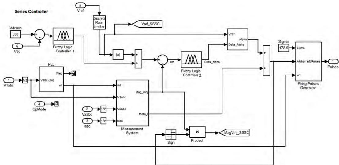
Fig. 2. FLC based series converter controller
