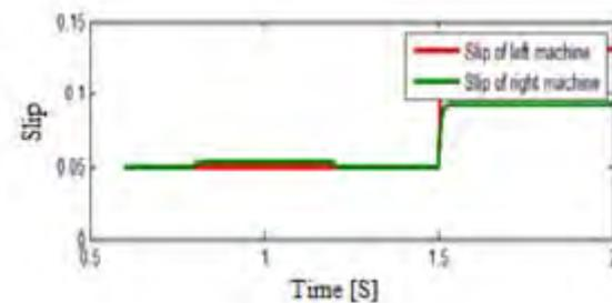
Figure. 7 (e) Slip rate of right and left side motor.
