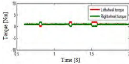
Figure. 7 (c) Torque waveform of right and left side motor.
