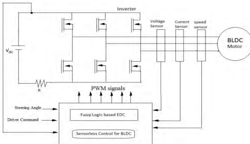
Figure 3. Fuzzy Logic based Electronic Differential Controller.
