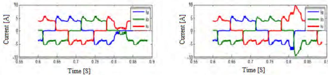
Figure.6(b) current waveform of right and left motor.
