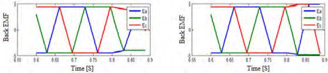
Figure. 6(d) Back EMF waveform of right and left motor.
