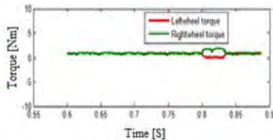
Figure.6(c) Torque waveform of right and left motor.
