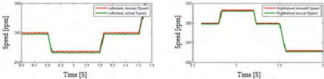
Figure 5(a) speed waveform of right and left side motor
