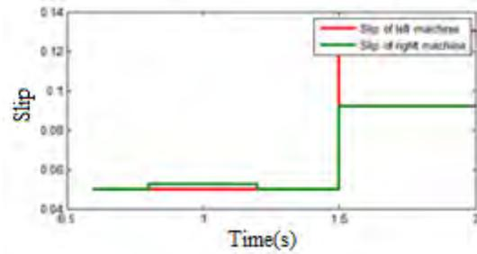
Figure 5(e) Slip rate of the left and right rear wheels
