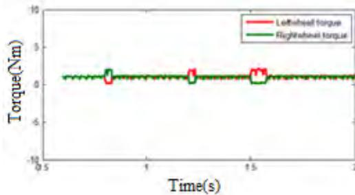
Figure.5(c) Torque waveform for right and left side motors
