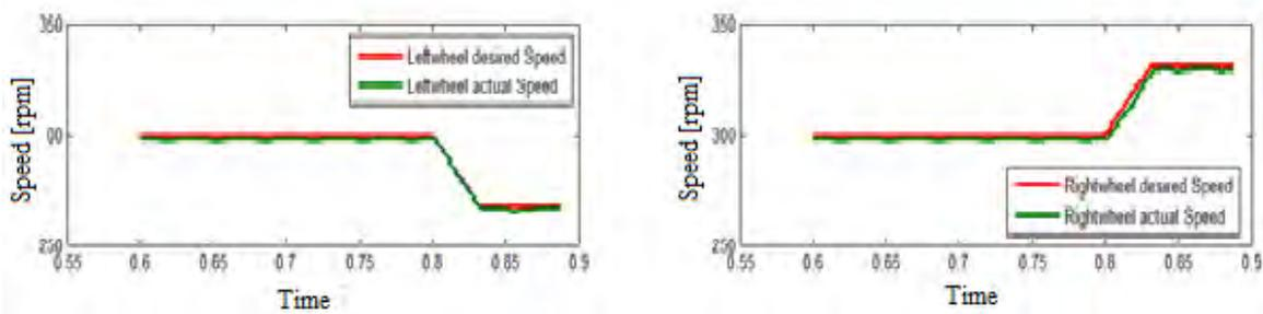
Figure.6(a) Speed waveform of right and left side motor.
