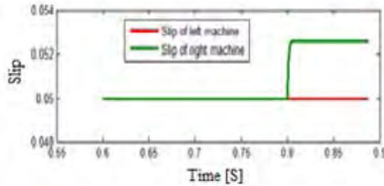
Figure 6(e) Slip rate of right and left motor.
