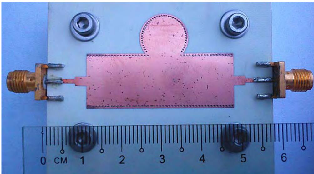
Fig. 12 Fabricated circular SIW bandstop filter
