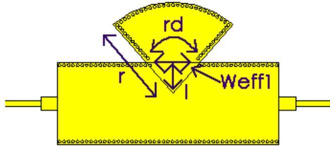
Fig. 3 Configuration of radial cavity resonator SIW bandstop filter
