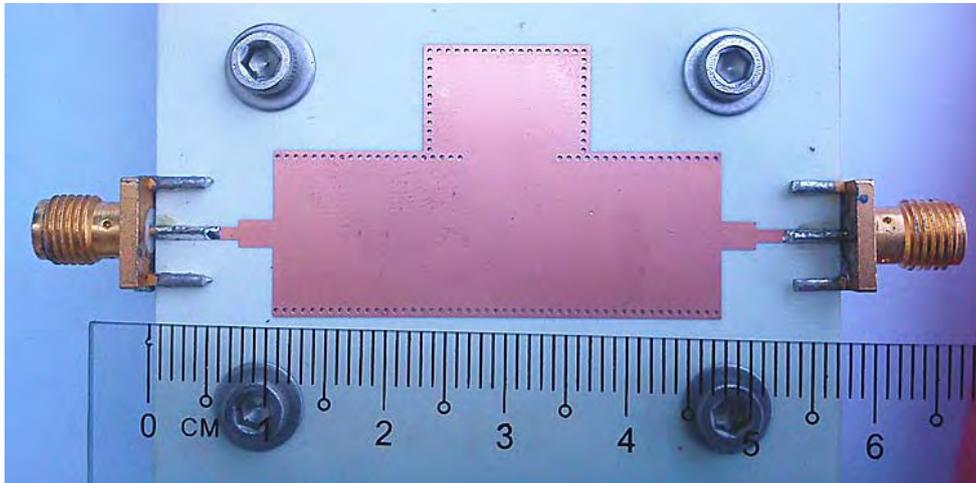
Fig. 11 Fabricated rectangular SIW bandstop filter
