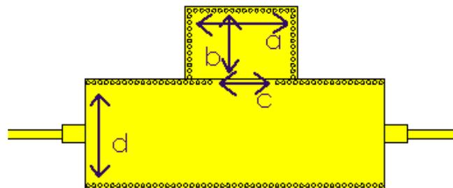
Fig. 1 Configuration of rectangular cavity resonator SIW bandstop filter
