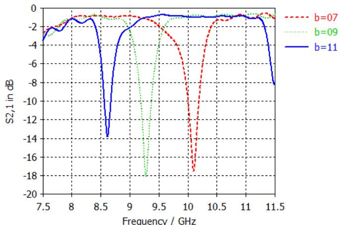
Fig. 5 Frequency response of variation of  $b$  for rectangular cavity resonator with dimension  $a=13.06\text{mm}$ ,  $c=8.3\text{mm}$ , and  $d=13.06\text{mm}$
