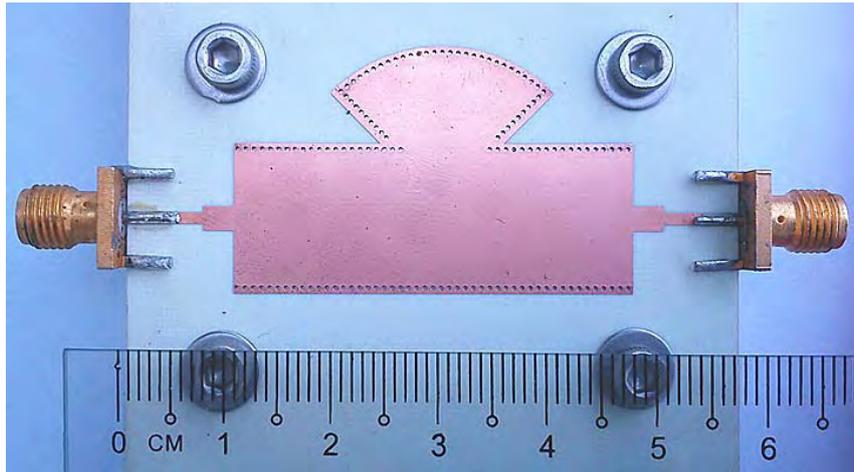
Fig. 13 Fabricated radial SIW bandstop filter
