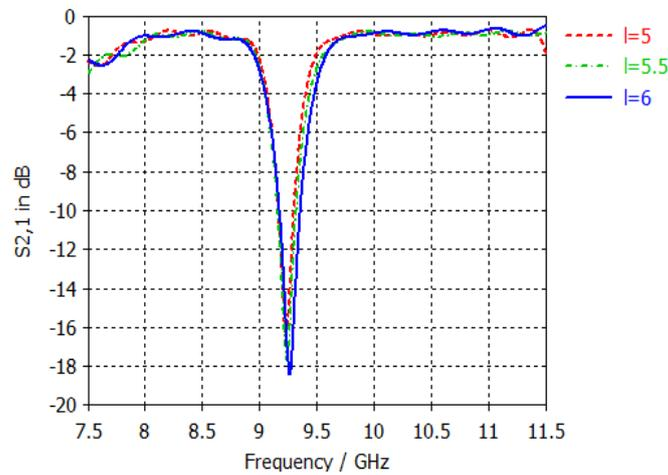
Fig. 10 Frequency response of variation of centre of radial cavity resonator with dimension  $rd=90^\circ$ ,  $r=14.7\text{mm}$ , and  $W_{eff}l=8.3\text{mm}$
