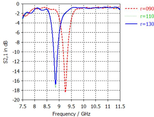
Fig. 8 Frequency response of variation of degree of radial cavity resonator with dimension  $r=14.7\text{mm}$ ,  $l=6\text{mm}$ , and  $W_{eff}l=8.3\text{mm}$
