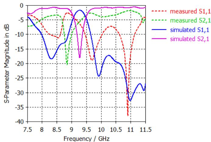
Fig. 14 Comparison between simulated and measured rectangular cavity resonator SIW bandstop filter
