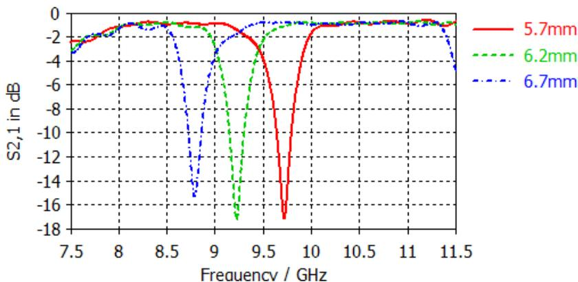
Fig. 6 Frequency response of variation of radius of circular cavity resonator with dimension  $a=8.3\text{mm}$ ,  $b=13.06\text{mm}$  and  $l=5\text{mm}$
