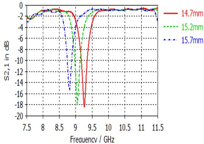
Fig. 9 Frequency response of variation of radius of radial cavity resonator with dimension  $rd=90^\circ$ ,  $l=6\text{mm}$ ,  $W_{eff}l=8.3\text{mm}$
