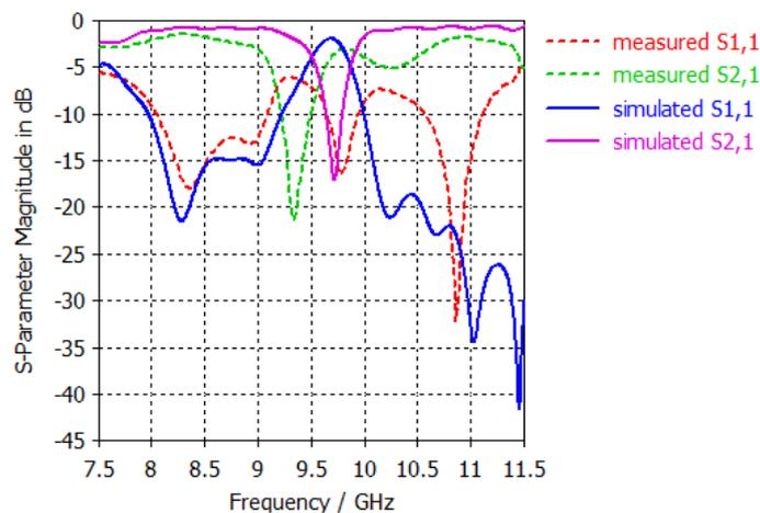
Fig. 15 Comparison between simulated and measured circular cavity resonator SIW bandstop filter
