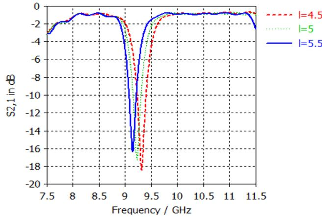
Fig. 7 Frequency response of variation of  $l$  of the circular cavity resonator with dimension of  $a=8.3\text{mm}$ ,  $b=13.06\text{mm}$ , and  $r=6.2\text{mm}$ .
