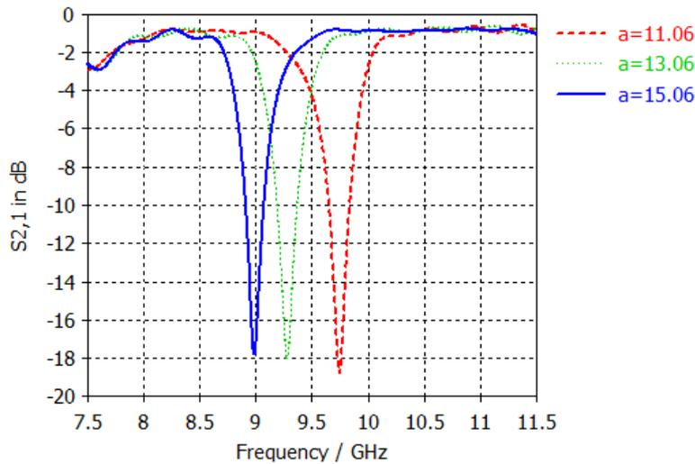
Fig. 4 Frequency response of variation of  $a$  for rectangular cavity resonator with dimensions  $b=9\text{mm}$ ,  $c=8.3\text{mm}$ , and  $d=13.06\text{mm}$
