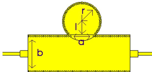
Fig. 2 Configuration of circular cavity resonator SIW bandstop filter
