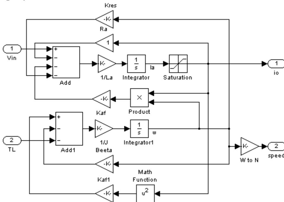
Fig 3. Simulink model of DC series motor
