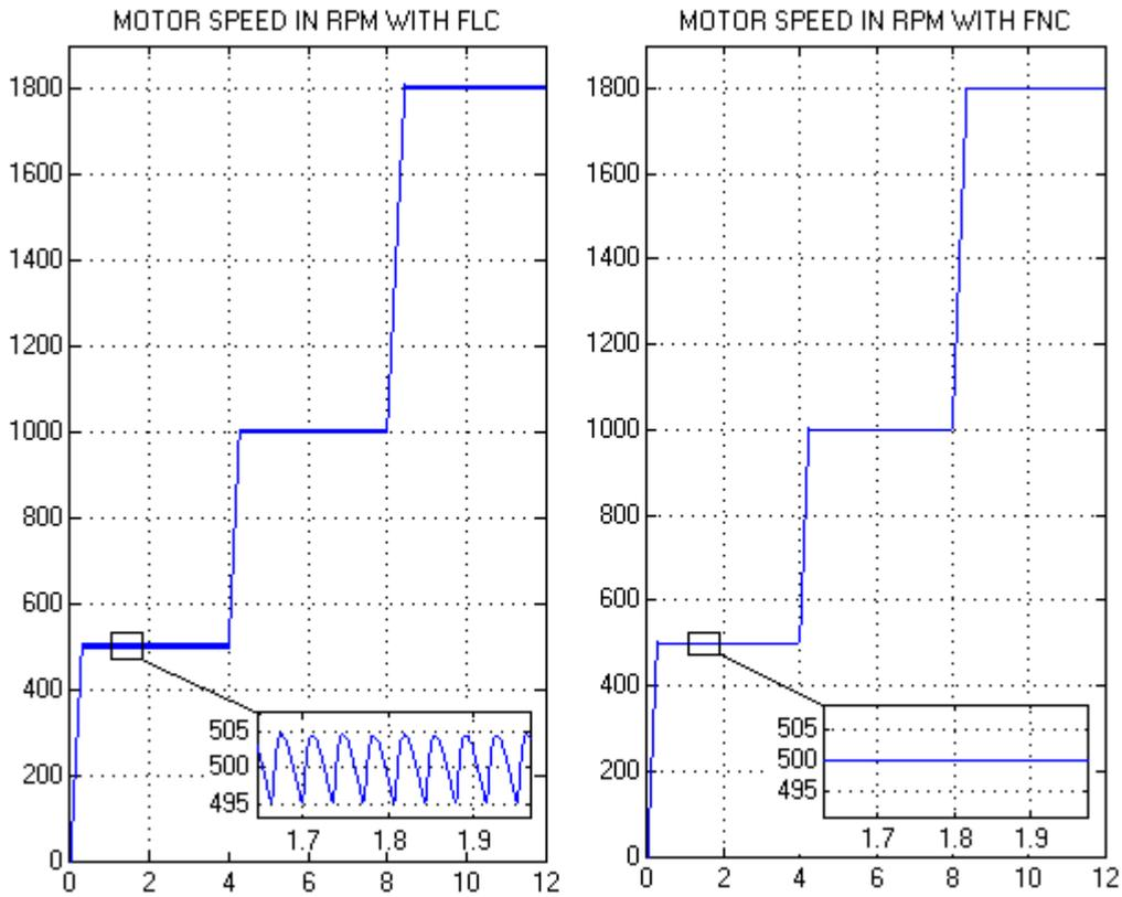
Fig. 14. Speed variation for the step change in reference speed at different interval with 10% load torque for DC series motor
