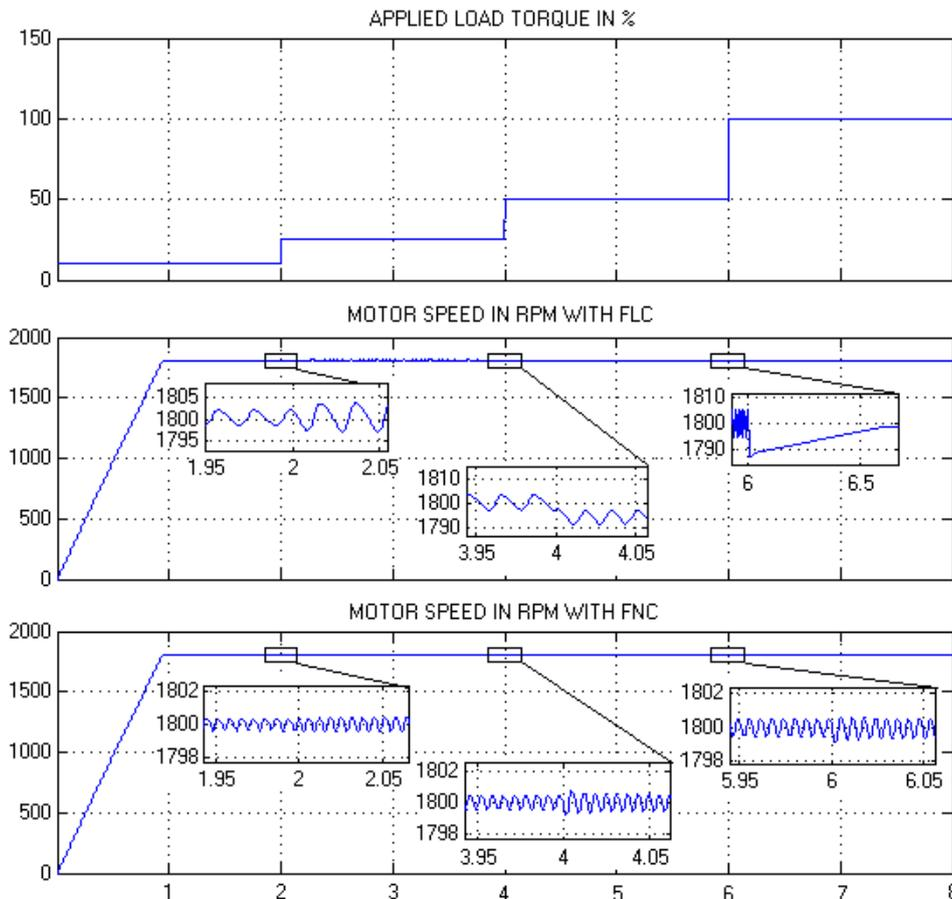
Fig. 16. Controller performance for load variation at different interval for rated speed with FLC and FNC for DC series motor
