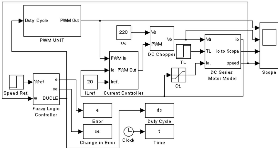
Fig 8. Simulink Model of the system with Fuzzy Logic Controller
