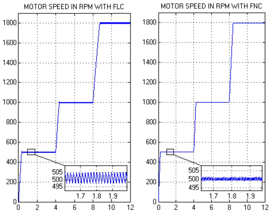
Fig. 15. Speed variation for the step change in reference speed at different interval with 10% load torque for DC Sep. Ext. Motor
