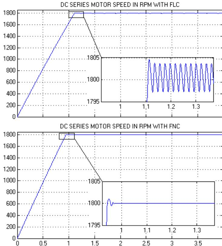
Fig. 12. Motor Speed variation with respect to time response for  $\omega_r=1800$ rpm for FLC and FNC with magnified view of settling part for DC series motor
