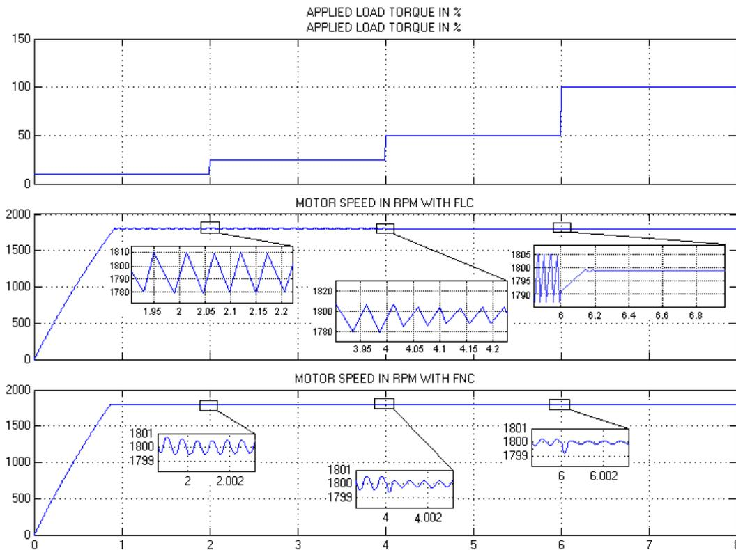
Fig. 17. Controller performance for load variation at different interval for rated speed with FLC and FNC for DC separately excited motor
