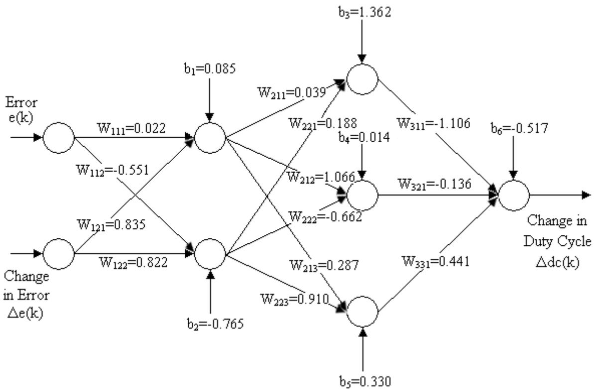
Fig. 10. Configuration of trained Neural Network
