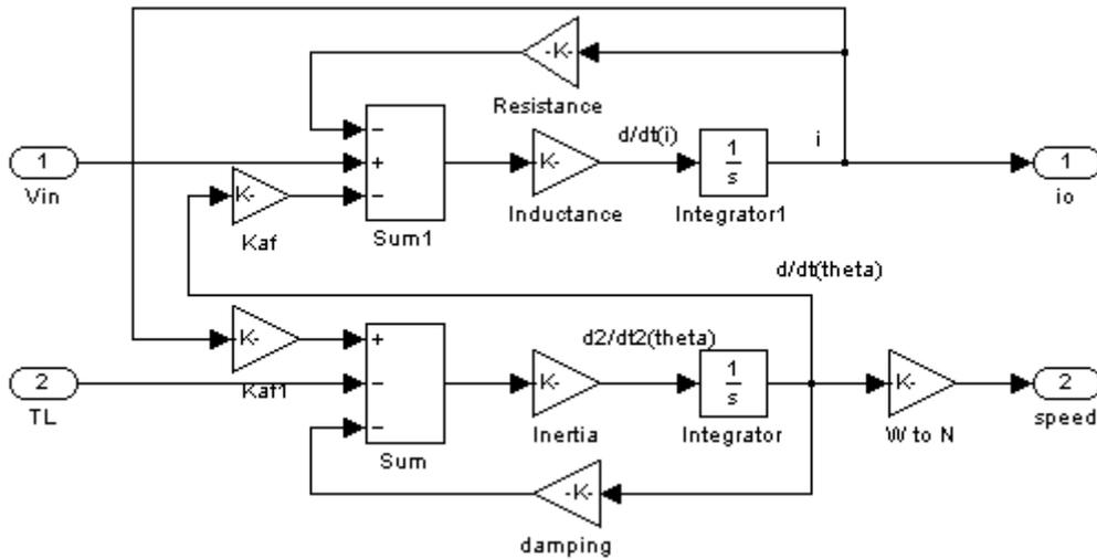
Fig 4. Simulink model of DC separately excited motor
