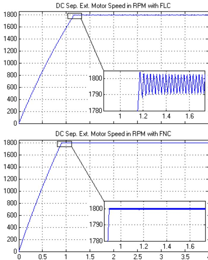
Fig.13 Motor Speed variation with respect to time response for  $\omega_r=1800$ rpm for FLC and FNC with magnified view of settling part for DC separately excited motor
