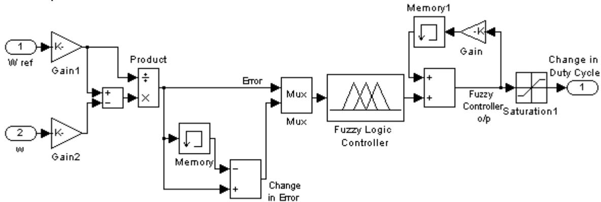
Fig 6. Structure of the fuzzy controller
