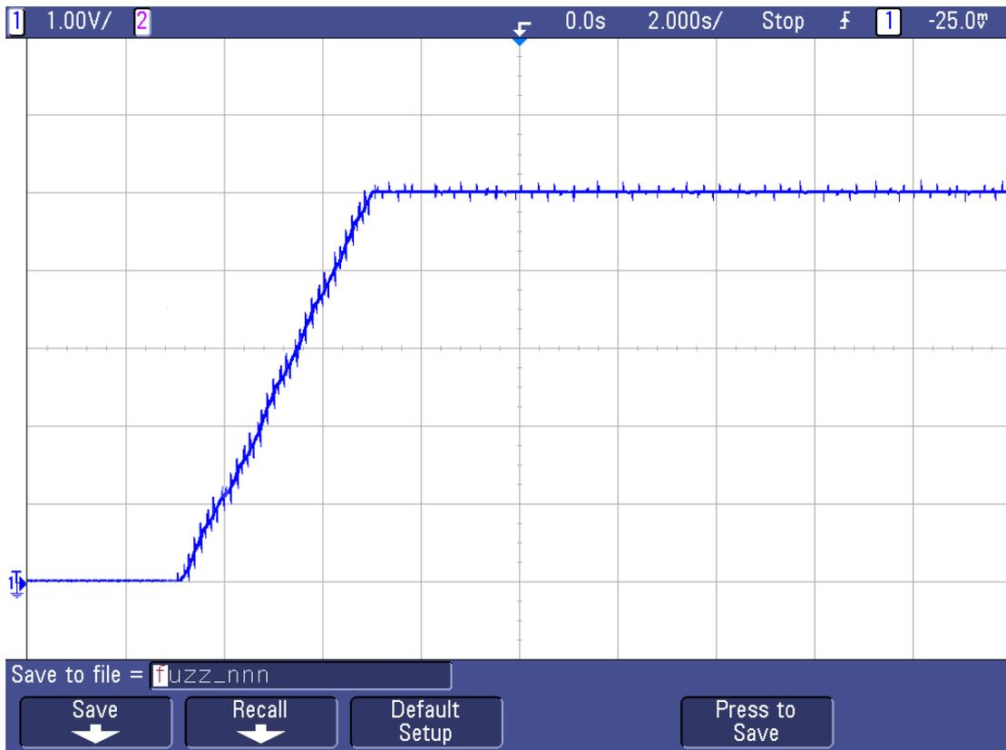
Fig.20. Experimental graph of speed variation for rated set speed using FNC for DC separately excited motor
