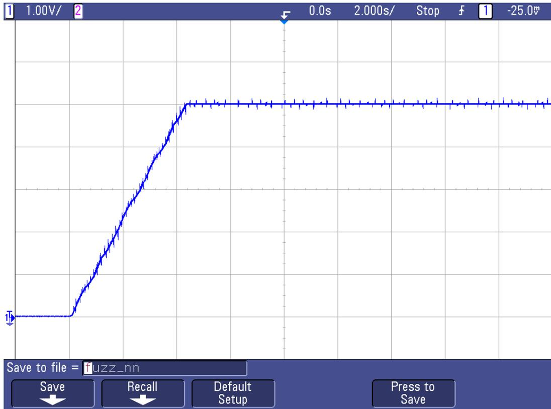
Fig.19. Experimental graph of speed variation for rated set speed using FNC for DC series motor
