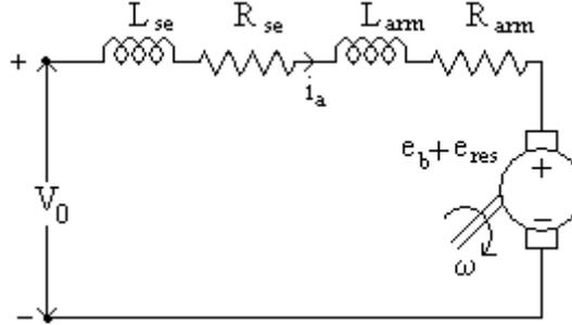
Fig 2. Equivalent Circuit of DC Series Motor
