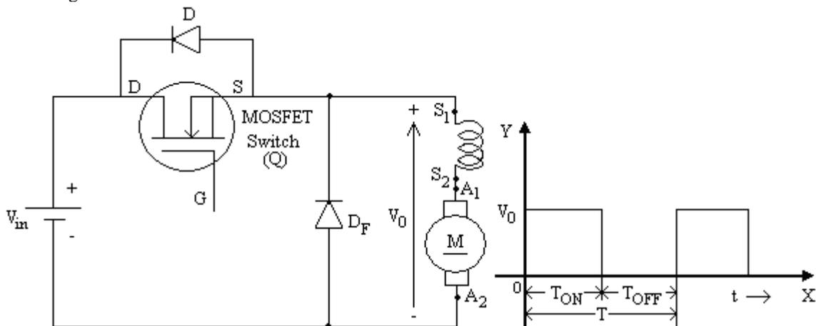
Fig 5. DC chopper circuit and waveform
