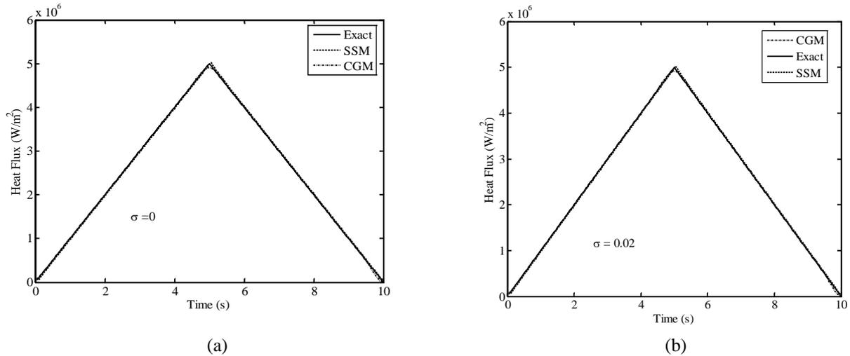
Fig. 5. Comparison of estimation of triangular heat flux using State Space Model (SSM) and Conjugate Gradient Model (CGM) for different measurement noise levels (a)  $\sigma = 0$  (b)  $\sigma = 0.02$
