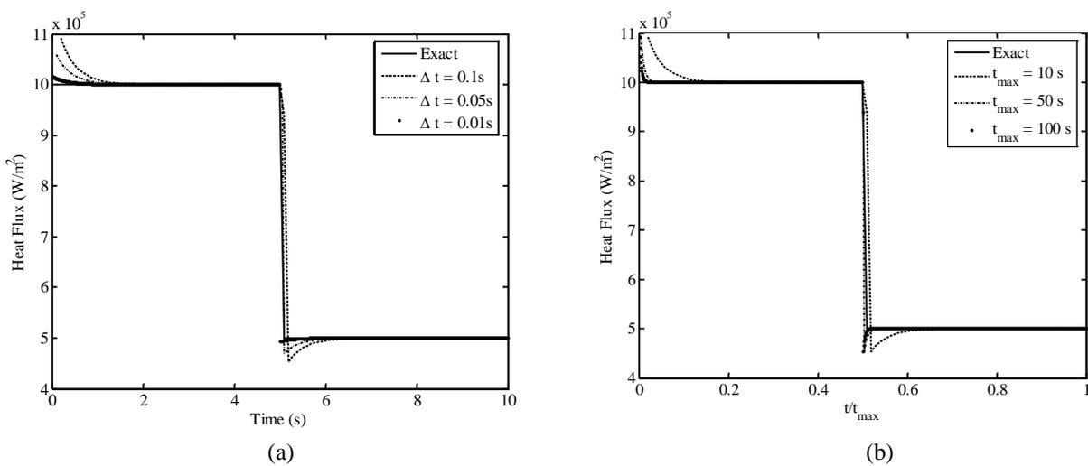
Fig. 2. Effect of (a) time step size and (b) pulse duration on estimation of step heat flux
