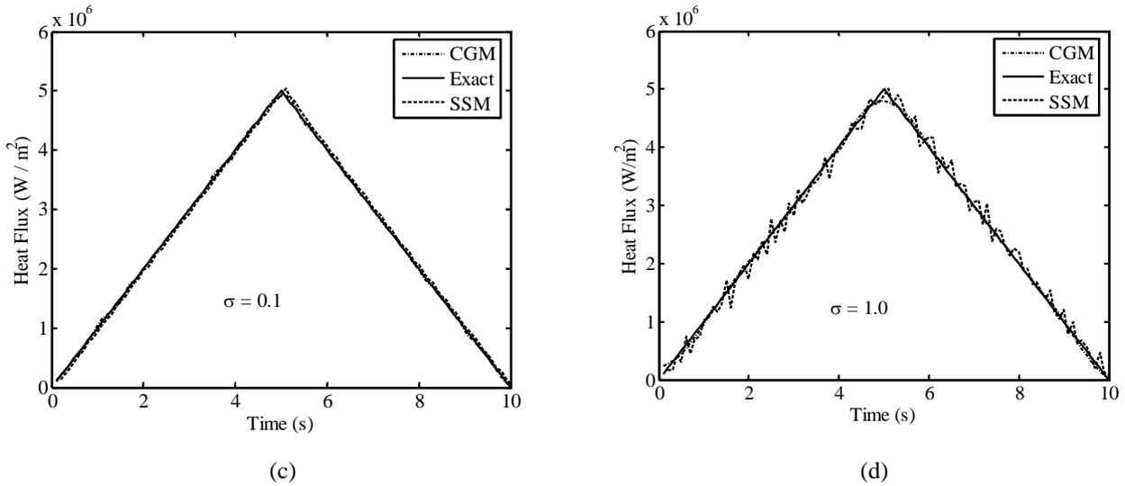
Fig. 5. Comparison of estimation of triangular heat flux using State Space Model (SSM) and Conjugate Gradient Model (CGM) for different measurement noise levels (c)  $\sigma = 0.1$  (d)  $\sigma = 1.0$
