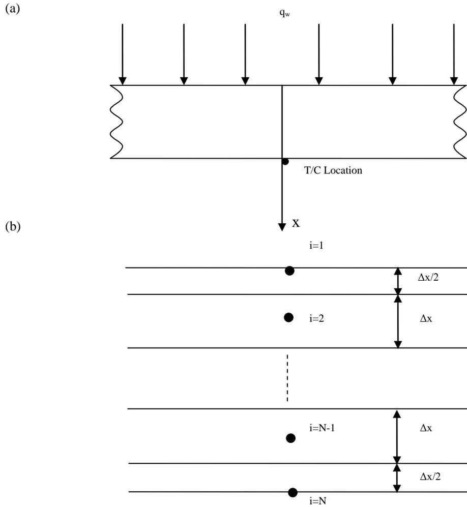
Fig. 1. (a) Schematic of the geometry and (b) discretisation scheme
