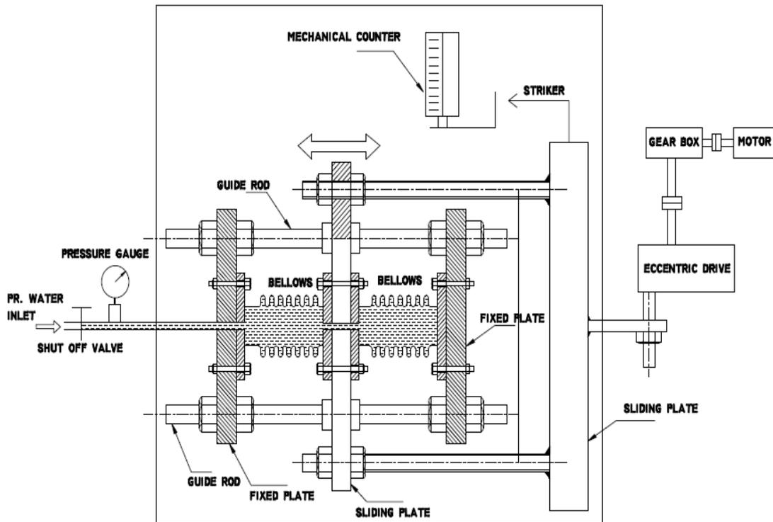
Fig. 6. Set up for Life Cycle Testing
