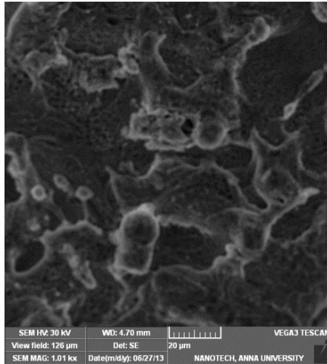
Fig. 7. Microstructure of parent metal of the tube
