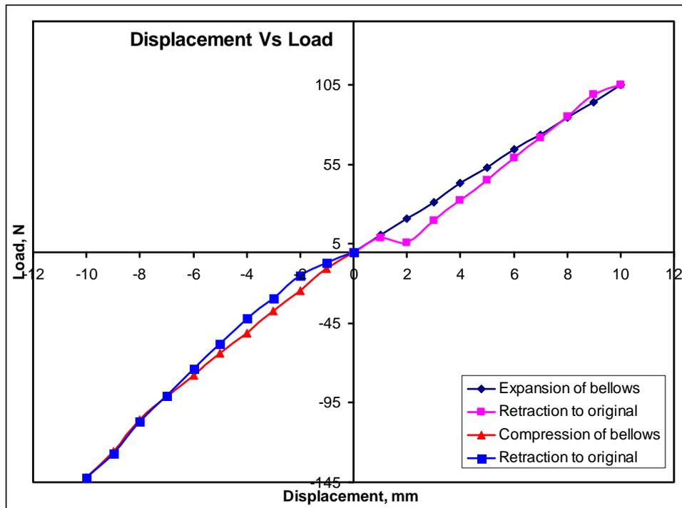
Fig. 5. Spring Rate of the Hydroformed bellows.
