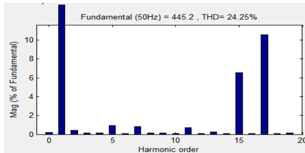
Fig. 22. Harmonic of the output line voltage by APODPWM for RL load
