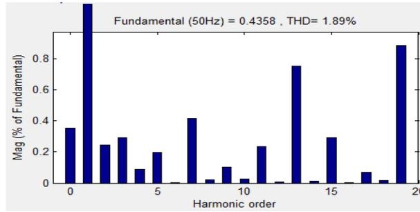
Fig. 17. Harmonic of the output line current by PODPWM for RL load
