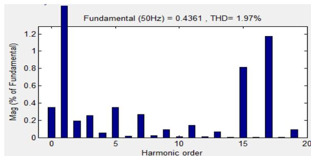
Fig. 23. Harmonic of the output line current by APODPWM for RL load
