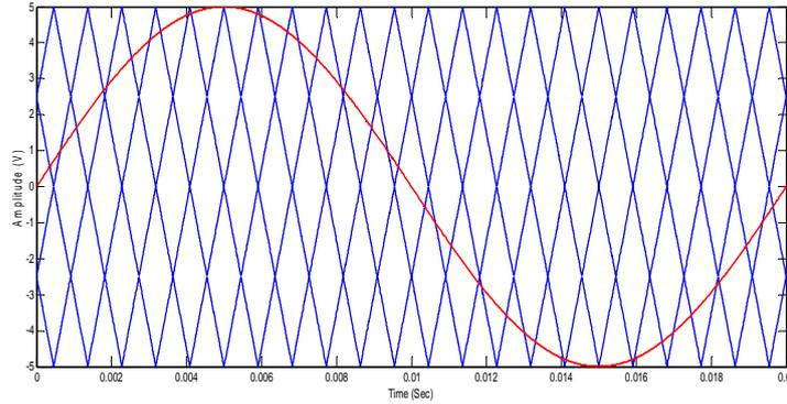
Fig. 4. Carrier arrangement for APODPWM strategy ( $m_a=1$  and  $m_f=23$ )
