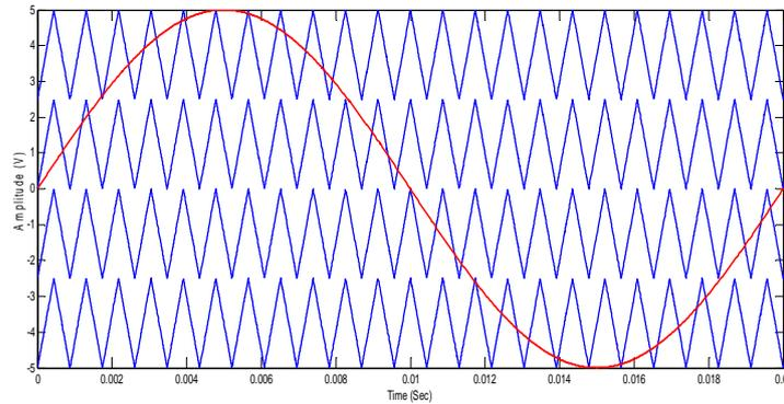
Fig. 2. Carrier arrangement for PDPWM strategy ( $m_a=1$  and  $m_f=23$ )
