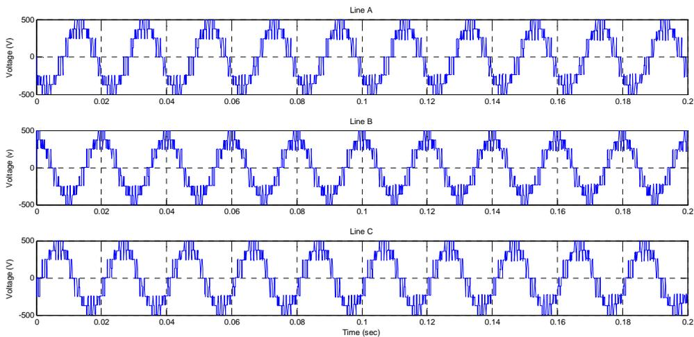
Fig. 19. Simulated line voltage by APODPWM for RL load
