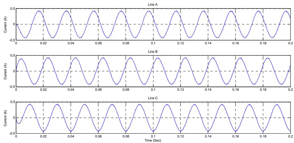
Fig. 26. Simulated line current by PSPWM for RL load
