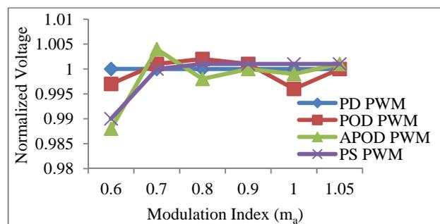
Fig. 30. Normalized phase voltage for different  $m_a$
