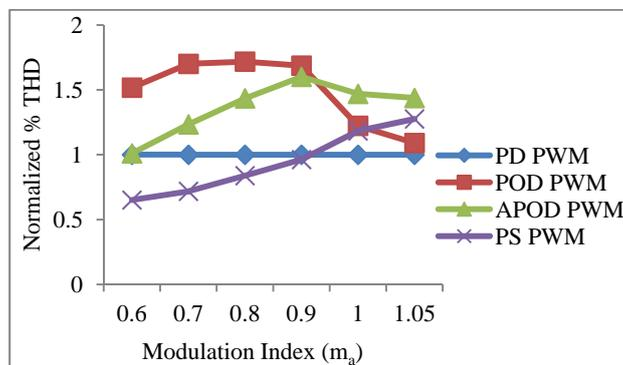
Fig. 35. % THD of line voltage for different  $m_a$
