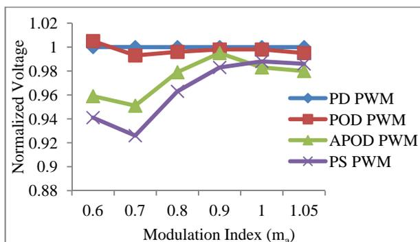
Fig. 32. RMS value of line voltage for different  $m_a$
