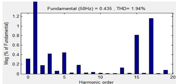
Fig. 29. Harmonic of the output line current by PSPWM for RL load
