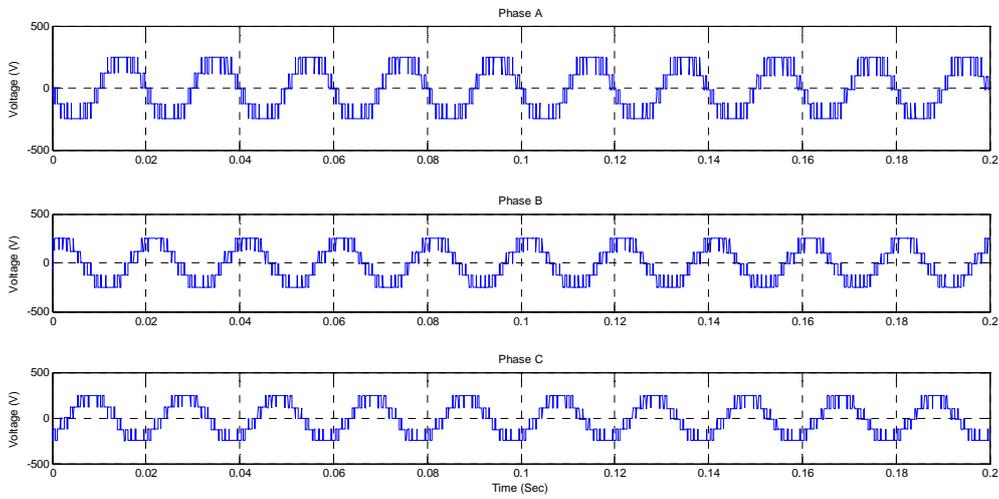
Fig. 18. Simulated phase voltage by APODPWM for RL load
