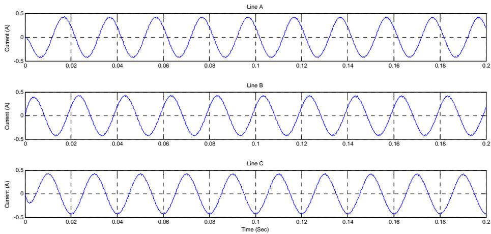
Fig. 8. Simulated line current by PDPWM for RL load
