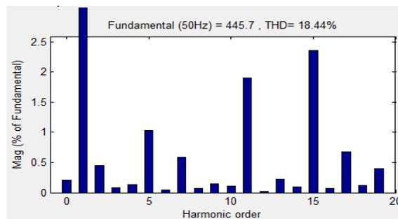
Fig. 16. Harmonic of the output line voltage by PODPWM for RL load
