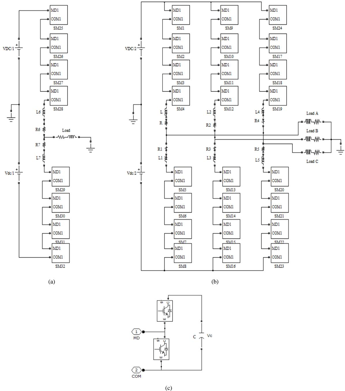
Fig. 1. (a) Single phase equivalent circuit of five-level modular multi-level inverter. (b) Three phase equivalent circuit of five-level modular multi-level inverter. (c). Bidirectional PWM chopper-cell with a floating dc capacitor.
