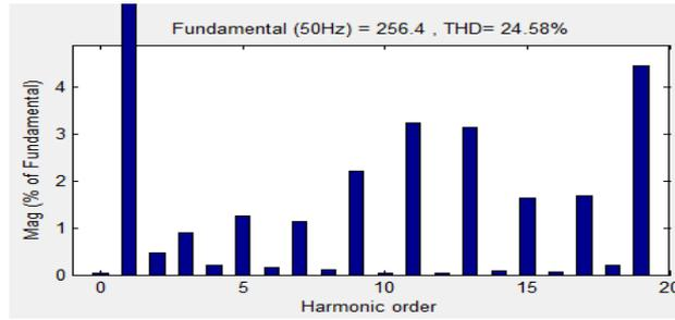
Fig. 9. Harmonic of the output phase voltage by PDPWM for RL load
