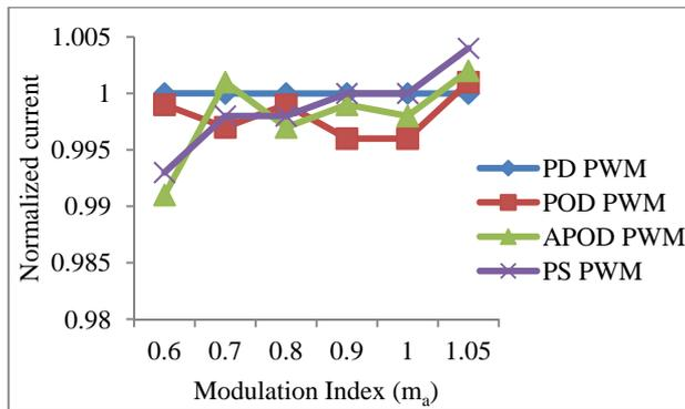
Fig. 33. Normalized line current for different  $m_a$
