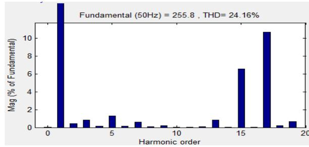
Fig. 27. Harmonic of the output phase voltage by PSPWM for RL load
