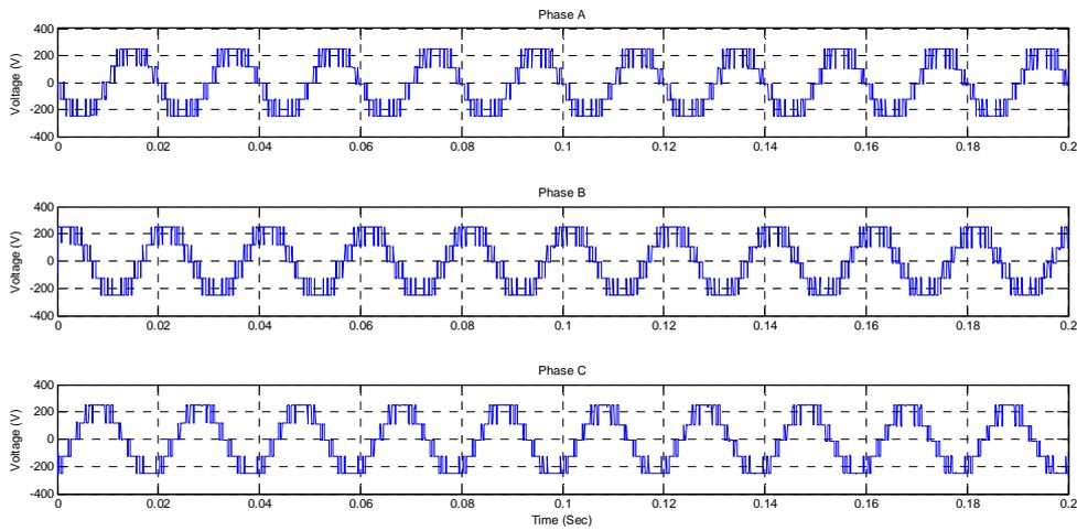
Fig. 6. Simulated phase voltage by PDPWM for RL load
