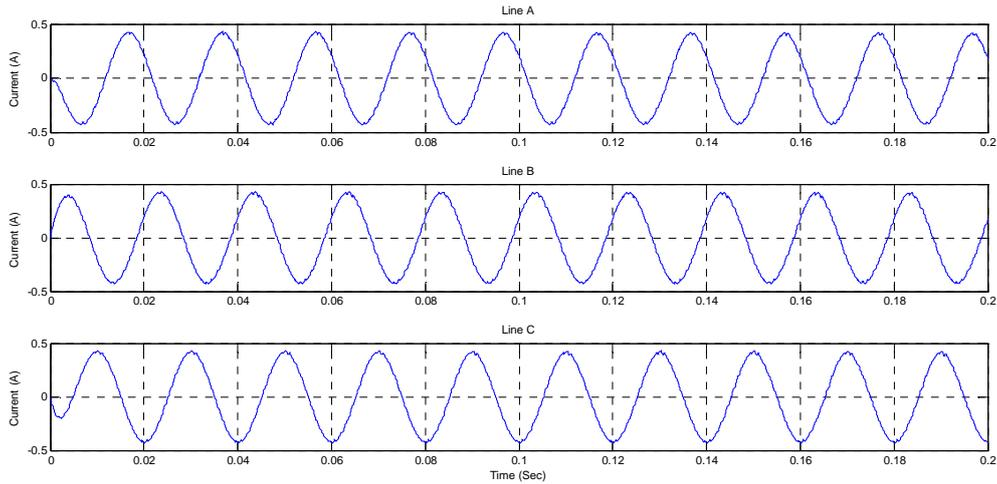
Fig. 20. Simulated line current by APODPWM for RL load
