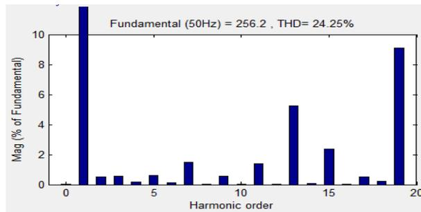
Fig. 15. Harmonic of the output phase voltage by PODPWM for RL load
