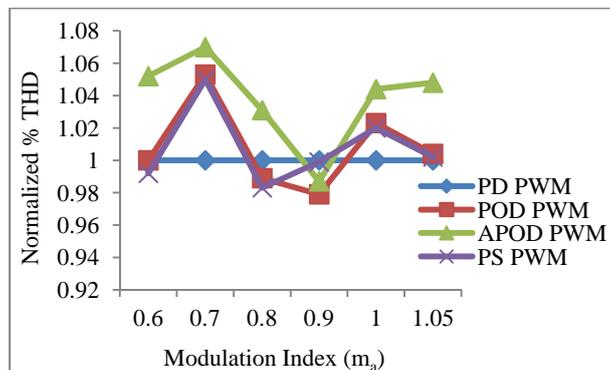
Fig. 34. % THD of Phase voltage for different  $m_a$
