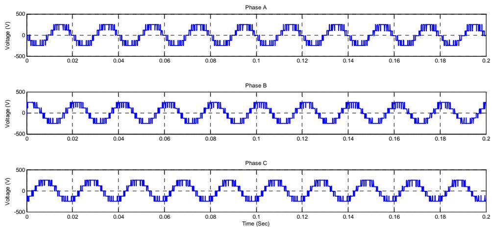
Fig. 12. Simulated phase voltage by PODPWM for RL load
