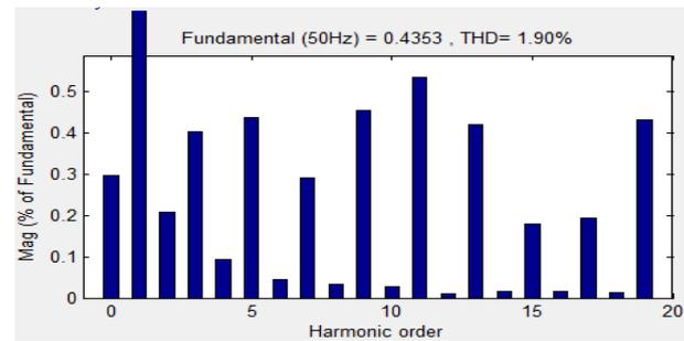
Fig. 11. Harmonic of the output line current by PDPWM for RL load
