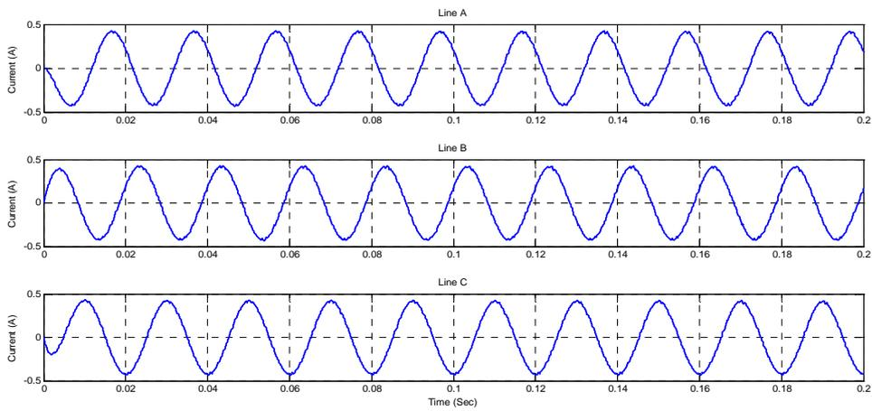
Fig. 14. Simulated line current by PODPWM for RL load
