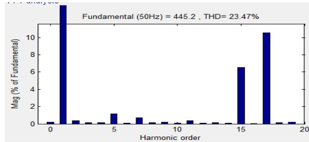
Fig. 28. Harmonic of the output line voltage by PSPWM for RL load
