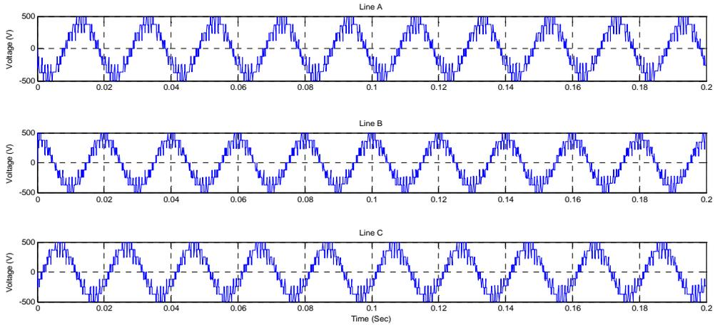
Fig. 13 Simulated line voltage by PODPWM for RL load
