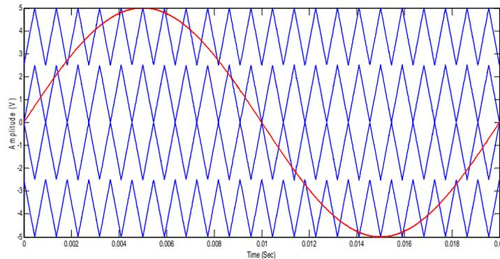
Fig. 3. Carrier arrangement for PODPWM strategy ( $m_a=1$  and  $m_f=23$ )
