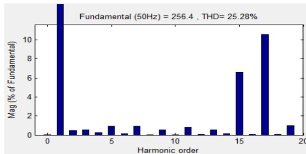
Fig. 21. Harmonic of the output phase voltage by APODPWM for RL load
