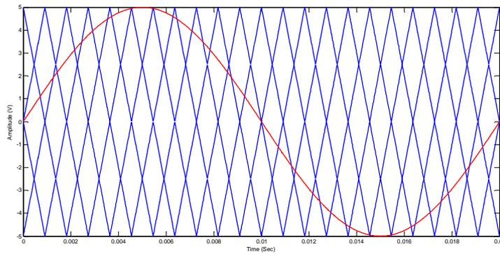
Fig. 5. Carrier arrangement for PSPWM strategy ( $m_a=1$  and  $m_f=23$ )
