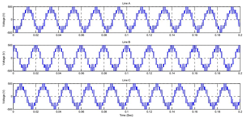
Fig. 25. Simulated line voltage by PSPWM for RL load
