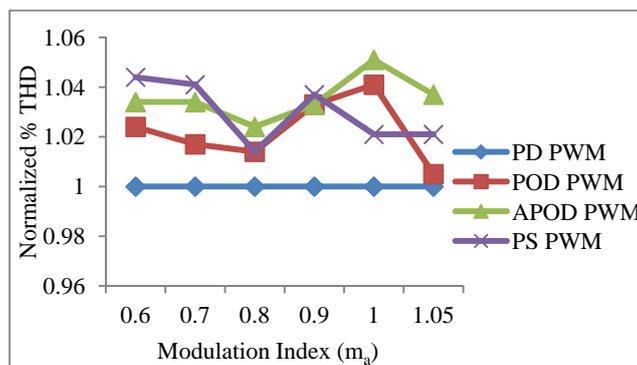
Fig. 36. % THD of line current for different  $m_a$
