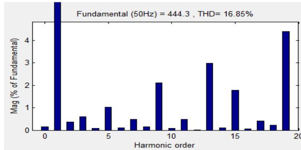
Fig. 10. Harmonic of the output line voltage by PDPWM for RL load
