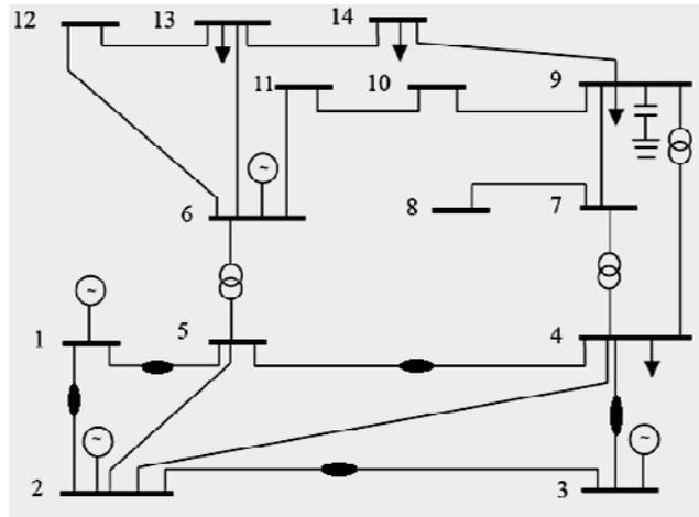
Fig.6. IEEE 14 bus system with 5 UPFC devices
