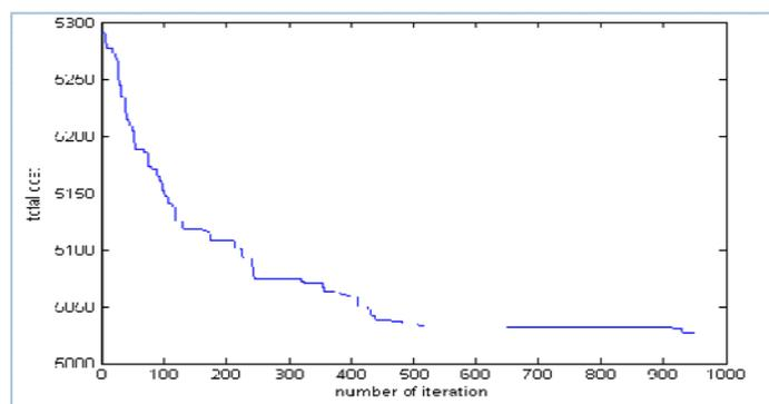
Fig.5.Total cost Vs Number of iteration curve for system with UPFC device in line 3-4
