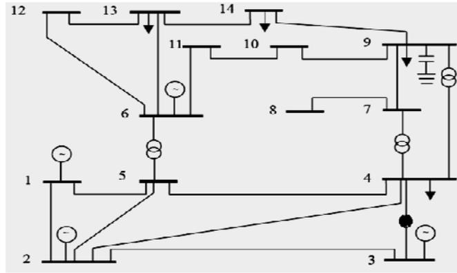
Fig.4. IEEE 14 bus system With UPFC device in line 3-4
