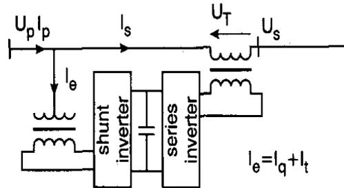
Fig.1. Schematic Lay Out Of UPFC
