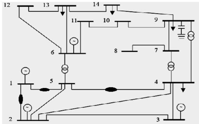
Fig.8. IEEE 14 bus system with 3 UPFC devices
