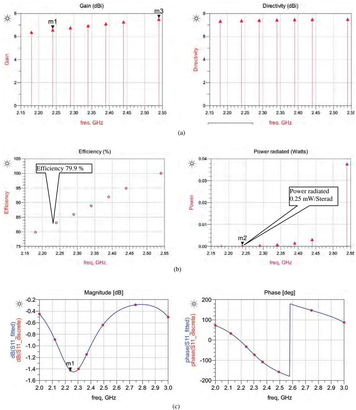
Fig. 5. Patch antenna performance parameters' visual representation (a) Gain and directivity (b) Efficiency and radiated power rates and (c) Return loss ( $S_{11}$  parameter) and phase reversals vs. frequency
