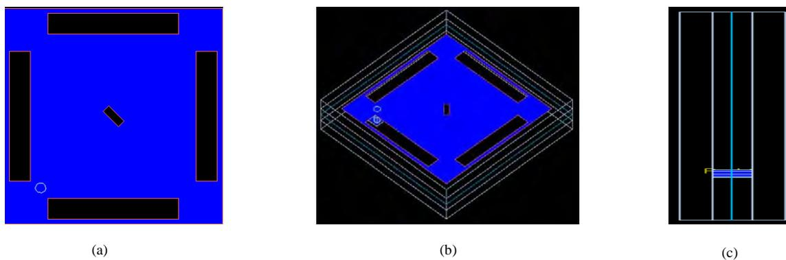
Fig. 2. Physical antenna design views (a) Top view of 4 slotted structure and feed location, (b) Isometric view of the same patch and (c) cross sectional view illustrating feed position across substrate.
