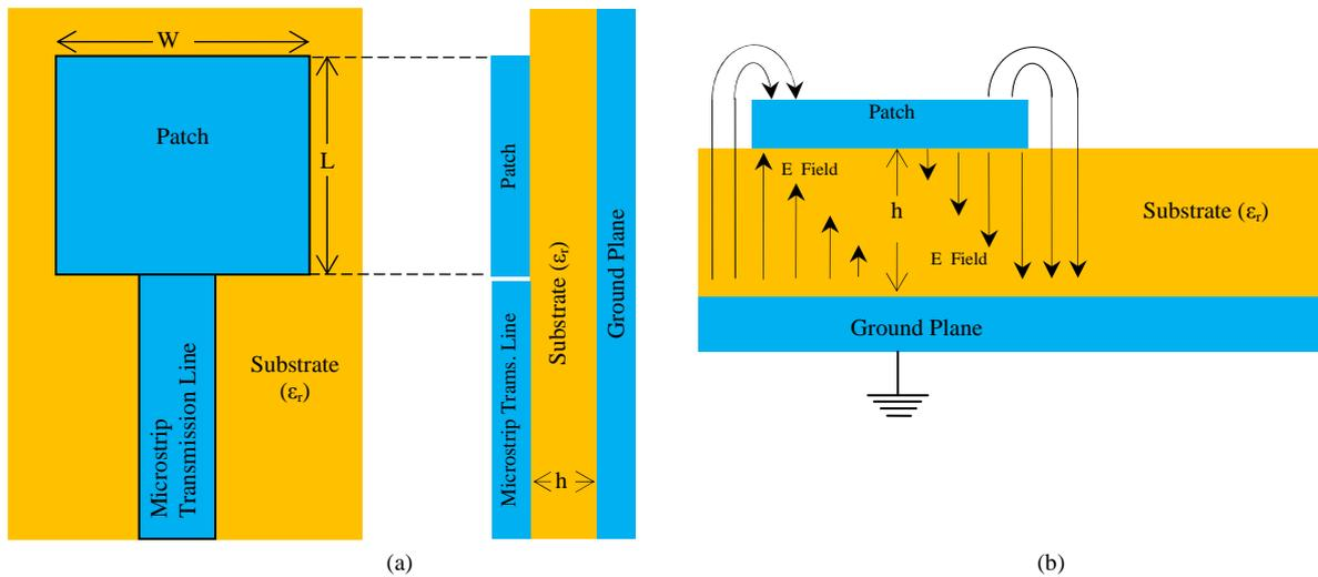
Fig. 1. Geometrical structure of a typical patch antenna (a) various dimensional presentation (b) Electrostatic Field distribution between patches and ground plane across the substrate
