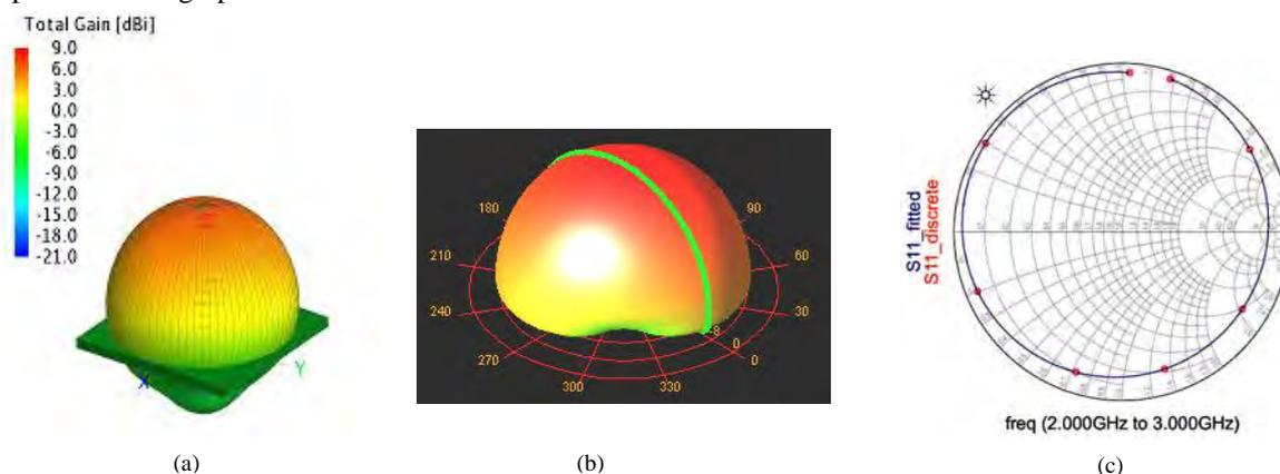
Fig. 3. Patch antenna performance parameters' visual representation (a) Directivity, gain magnitude and reference direction, (b)  $\phi$  ( $\varphi$ ) model representation (c) Impedance matching representation on Smith chart
