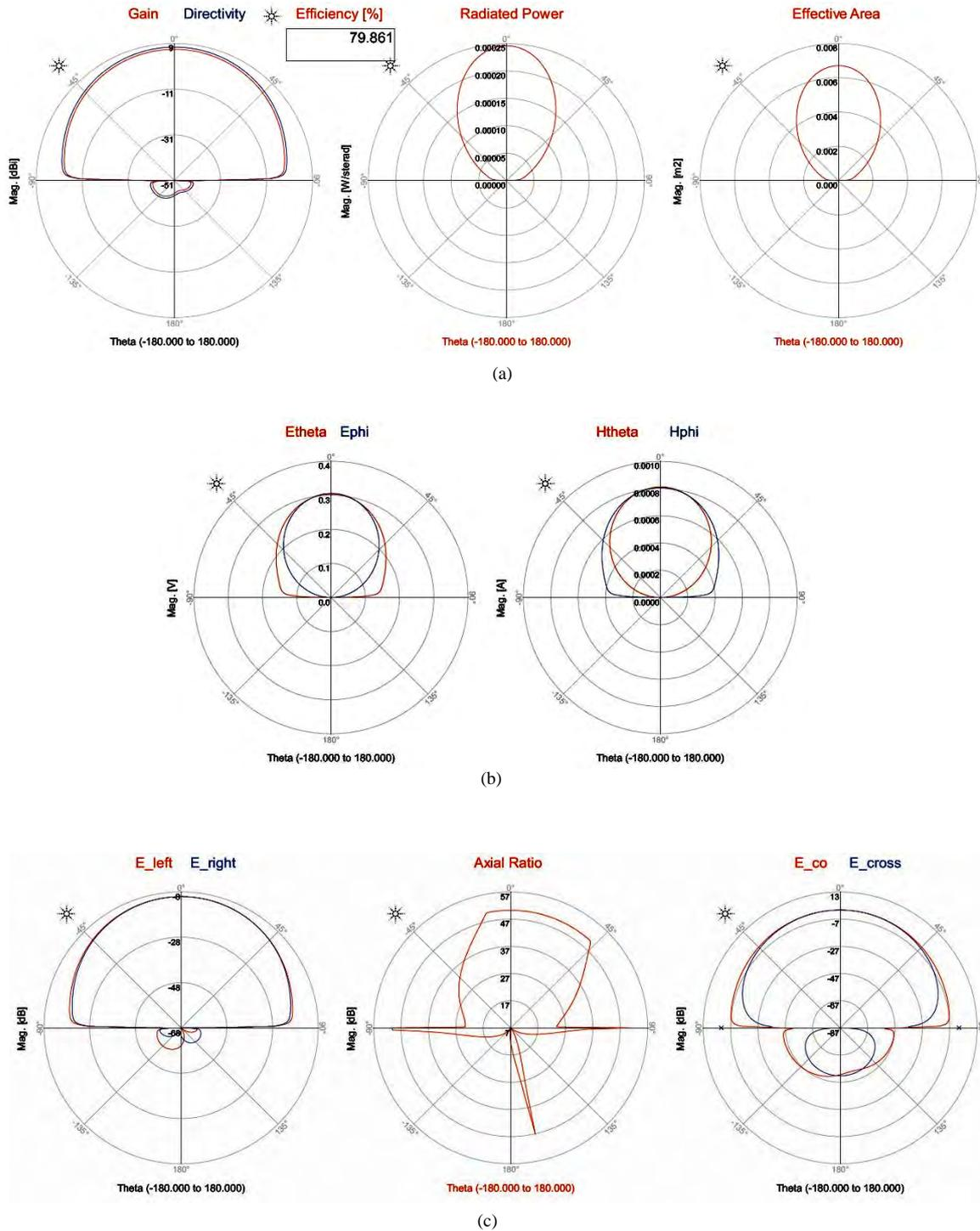
Fig. 4. Patch antenna performance parameters' visual representation (a) Gain vs. directivity, radiated power and effective area (b) Absolute fields and (c) Circular polarization, axial ratio and linear polarization pattern
