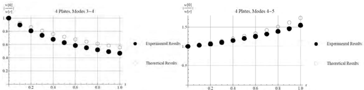
Fig. 3 Displacement ratios for four plates, coupled modes: 3-4 and 4-5
