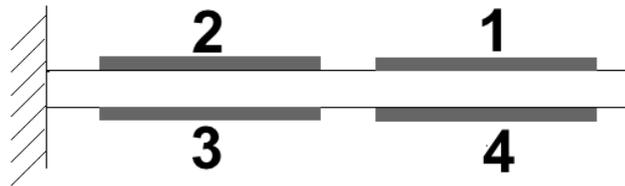
Fig. 2 PZT's plates configuration
