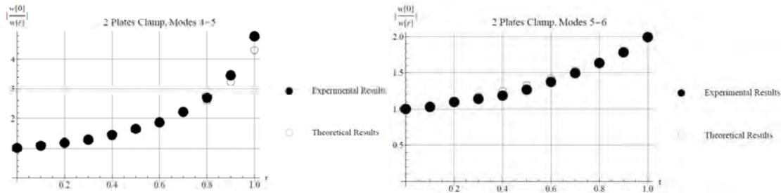
Fig. 4 Displacement ratios for two plates near the clamp: coupled modes: 4-5 and 5-6
