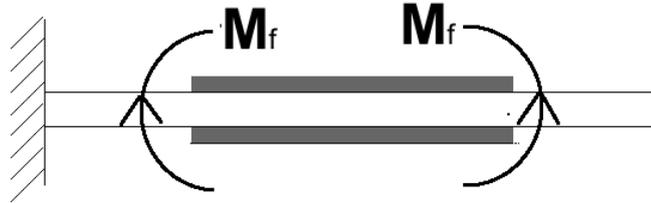
Fig. 1 Reference configurations and flexural moments applied by piezoelectric plates (Pin Force Model)
