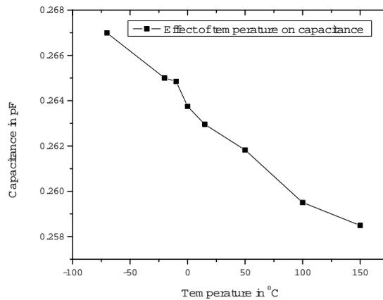
Fig.8. Effect of temperature on capacitive sensitivity.
