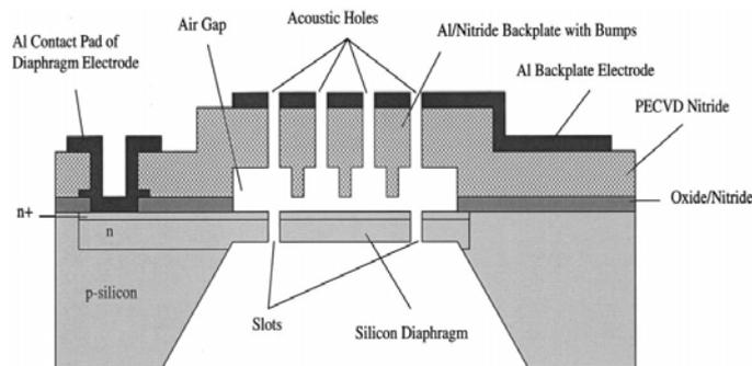
Fig. 9. Cross section of slotted silicon microphone (adapted from [46]).
