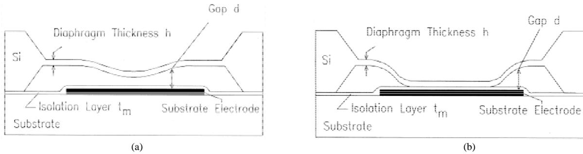
Fig.3. Schematic diagram of principle of Touch mode pressure sensor (a) Normal mode operation (b) Touch mode operation (adapted from [21]).
