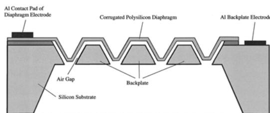
Fig. 11. Cross section of corrugated silicon microphone (adapted from [46]).
