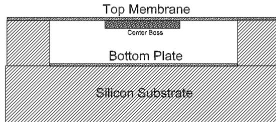
Fig.4. Schematic diagram of bossed diaphragm capacitive pressure sensor [29].
