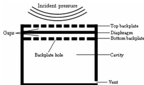
Fig. 10. Models of a dual backplate capacitive MEMS microphone physical model (adapted from [49]).
