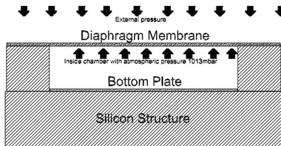
Fig.5. Schematic diagram of principle of CDPS Structure (adapted from [26]).
