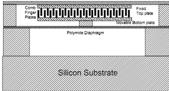
Fig.6. Schematic diagram of CDPS comb plate Structure (adapted from [31]).
