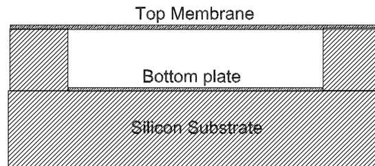
Fig.2. Schematic diagram of capacitive pressure sensor structure (adapted from [31]).
