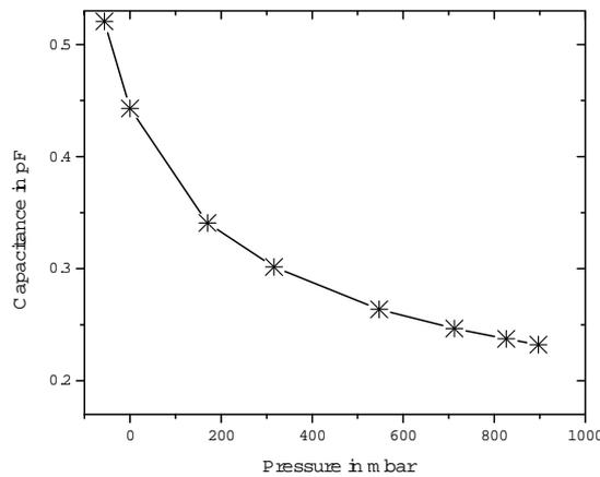
Fig.7. Characteristics of Pressure Vs Capacitance (C-P).
