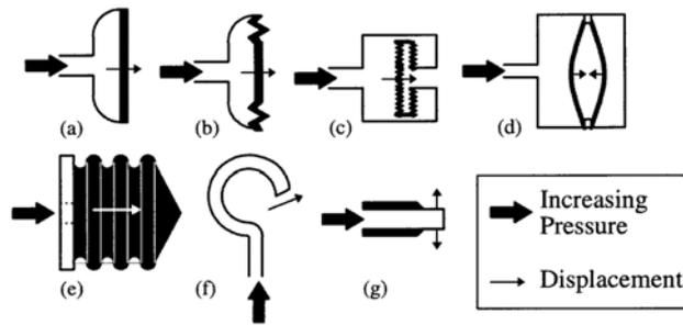
Fig. 1. Macroscopic pressure sensors : (a) simple diaphragm, (b) corrugated diaphragm, (c) capsule, (d) capacitive sensor, (e) bellows, (f) Bourdon tube, (g) straight tube (adapted from [1]).
