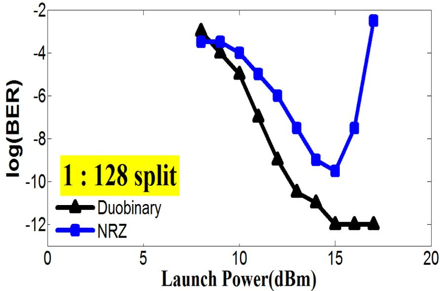
Fig. 6. Downstream signal transmission result for duo binary and NRZ with 1:128 split ratio over corning nexcore SMF-28e+ fiber
