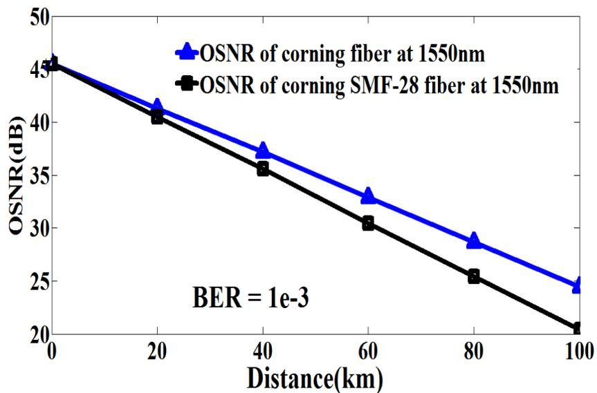
Fig. 5. Distance vs osnr over both fibers
