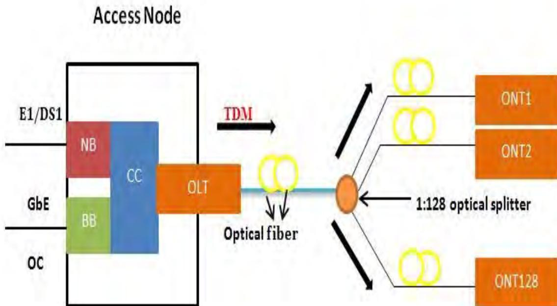
Fig. 3. Downstream transmission of TDM-PON architecture
