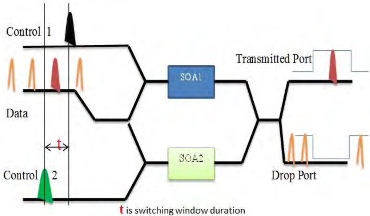
Fig. 4. Demultiplexing of channels by using two SOAs
