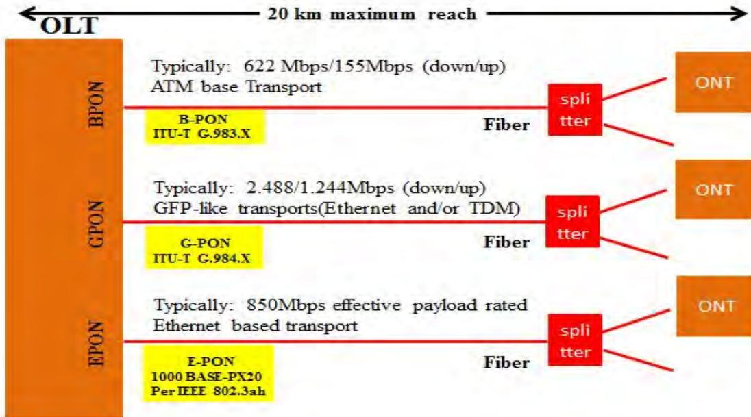
Fig. 1. TDM-PON architecture and Technologies
