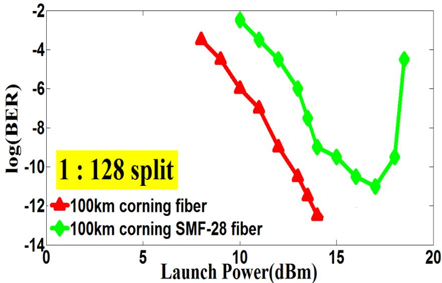
Fig. 7. Downstream signal transmission result for duo binary with 1:128 split ratio over both fibers
