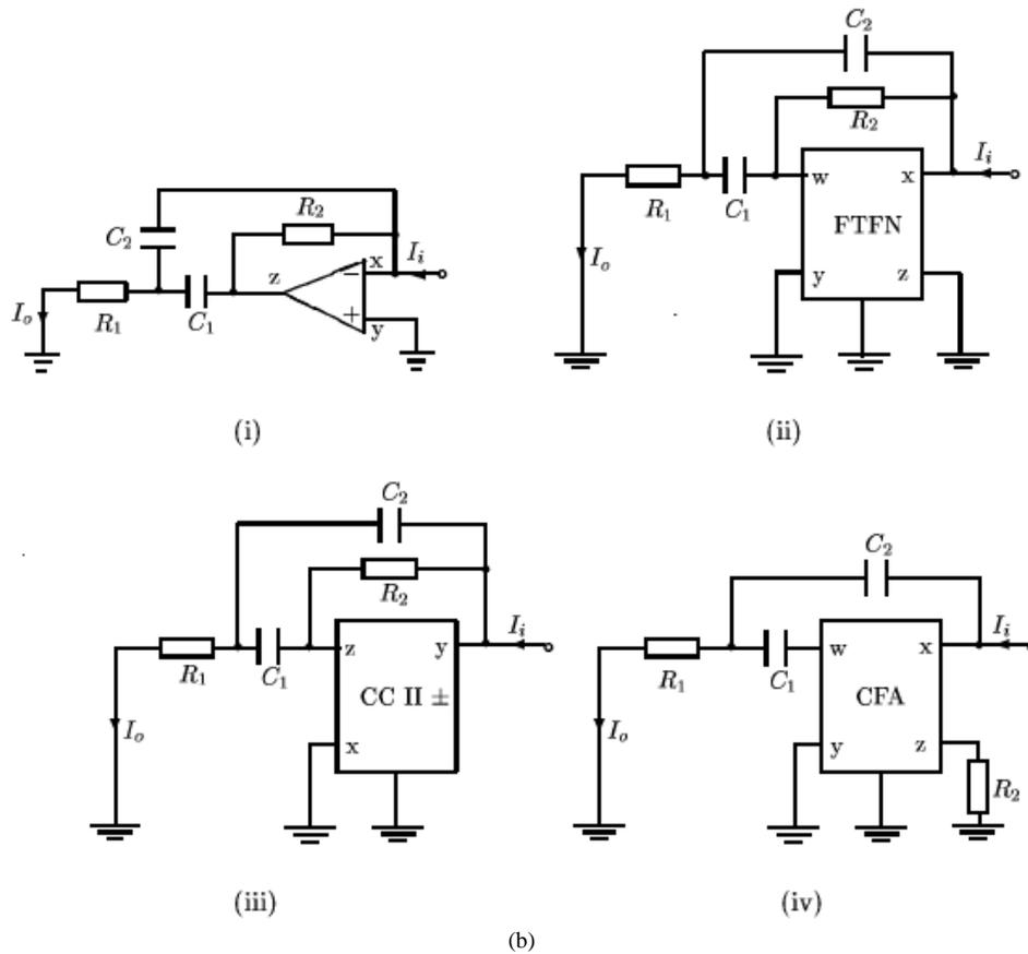
Fig. 19. (a) OA based VM band-pass filter and (b) four CM band-pass filters.
