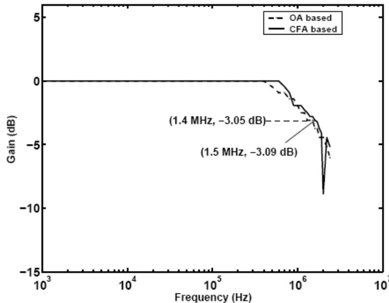
Fig. 22. Experimental results – Frequency responses of low-pass filters shown in Fig. 15 with  $R = R_1 = 1 \text{ k}\Omega$ ,  $C = 100 \text{ pF}$  for  $f_0 = 1.59 \text{ MHz}$ .
