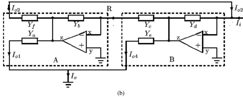
Fig. 6. (a) Loobering VM OA circuit and (b) CM OA circuit.
