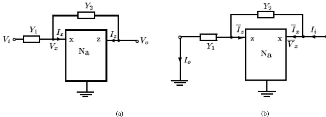
Fig. 1. (a) VM circuit and (b) CM circuit.
