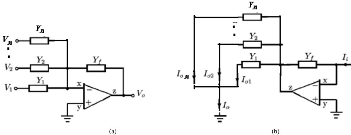
Fig. 5. OA-based (a) multi-input VM circuit and (b) multi-output CM circuit.
