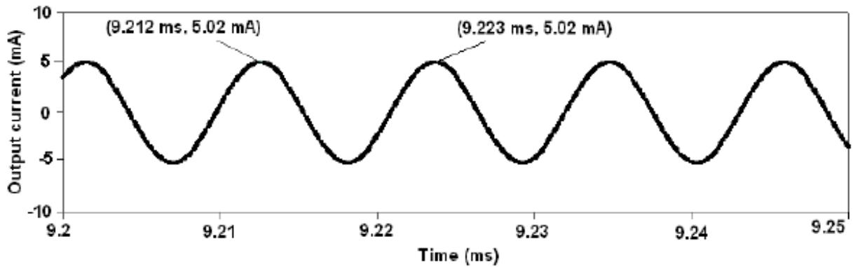
Fig. 21.  $I_o$  waveform of the phase shift oscillator with  $R = 649.74 \Omega$ ,  $C = 1$  nF,  $R_f = 25$  k $\Omega$ .
