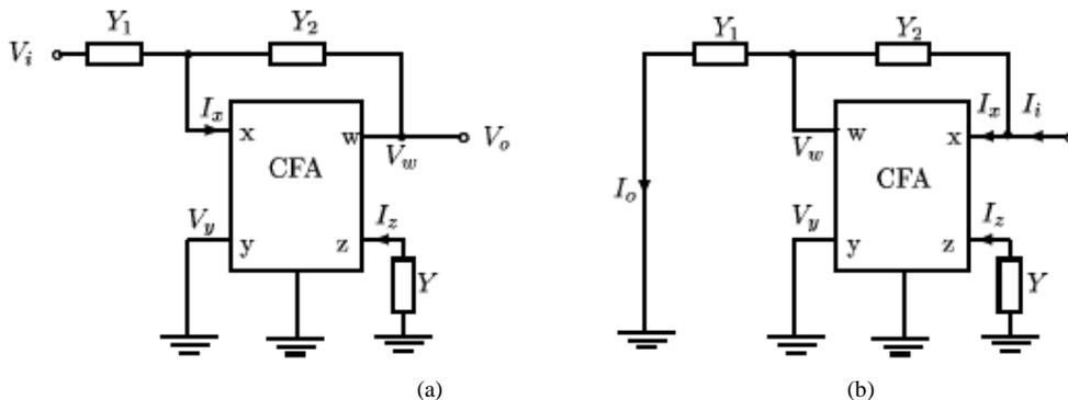
Fig. 9. CFA-based (a) VM and (b) CM circuits.
