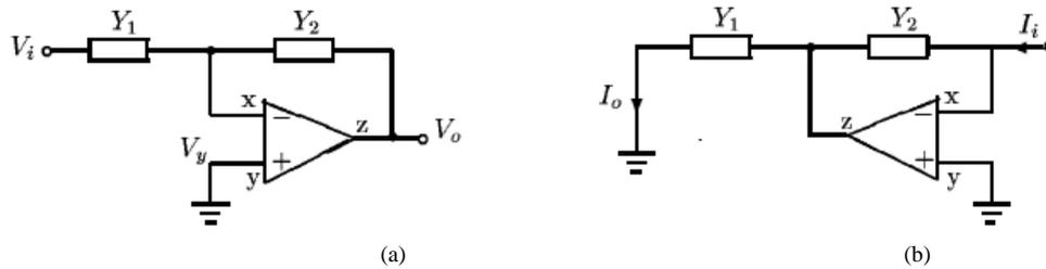
Fig. 2. OA-based (a) VM circuit and (b) CM circuit.
