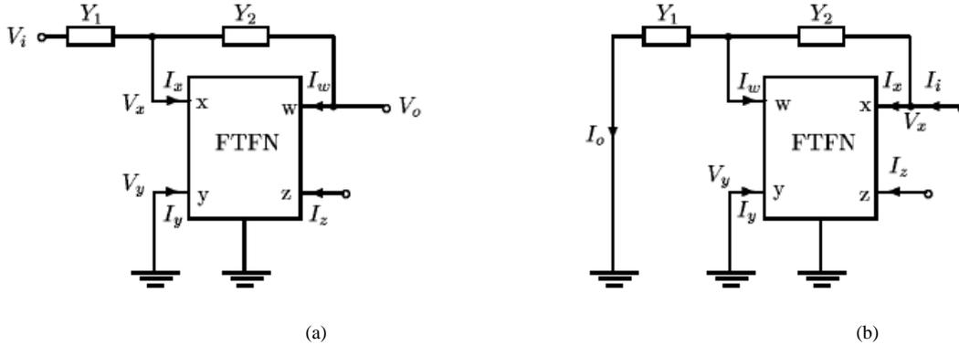
Fig. 3. FTFN-based (a) VM circuit and (b) CM circuit.
