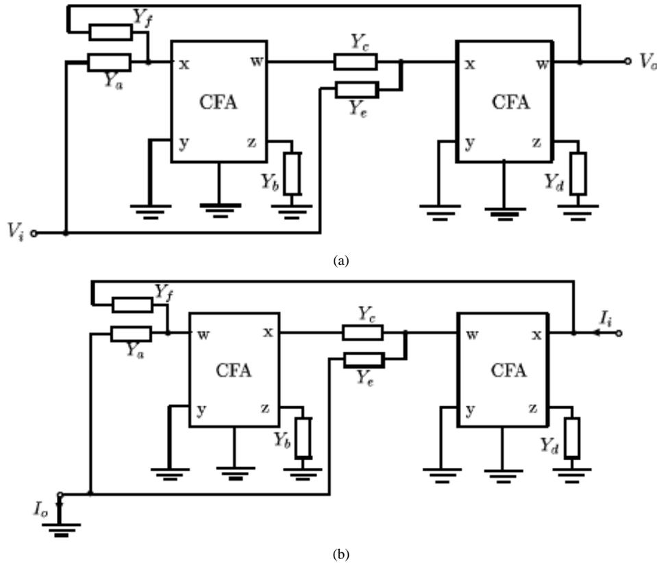
Fig. 10. (a) VM and (b) CM circuits with more number of CFAs.
