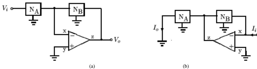
Fig. 13. Generalized OA based (a) VM and (b) CM circuits with 3 terminal passive network.
