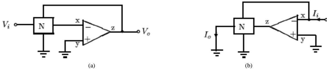
Fig. 18. Generalized OA based (a) VM and (b) CM circuits with 4 terminal passive network.
