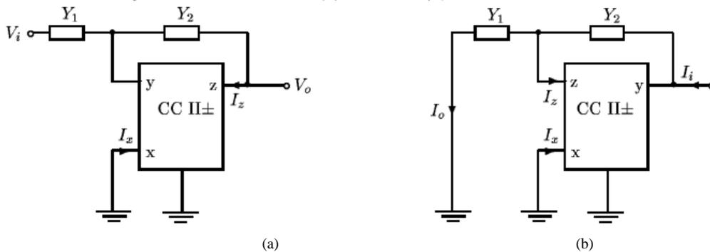
Fig. 4. CCII-based (a) VM circuit and (b) CM circuit.
