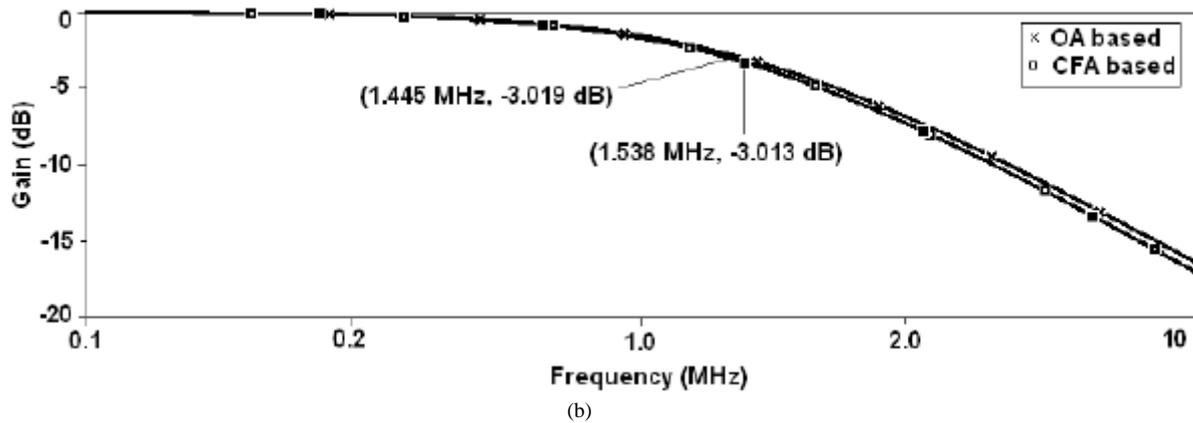
Fig. 20. Simulation results: Frequency responses of the low-pass filters for  $f_0 = 15.9$  kHz and (b) for  $f_0 = 1.59$  MHz.
