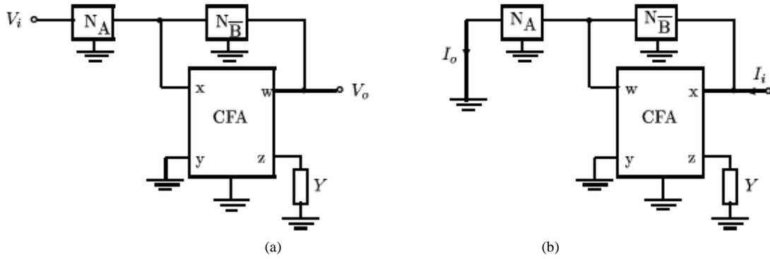
Fig. 14. Generalized CFA based (a) VM and (b) CM circuits.
