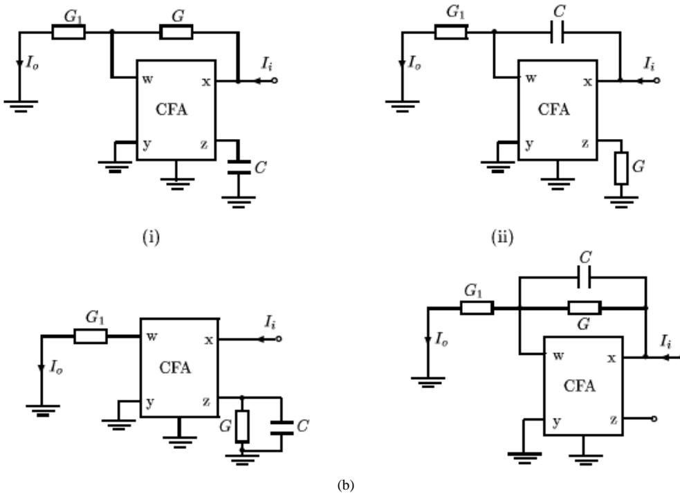
Fig. 15. (a) OA based VM low-pass filter and (b) four CFA based CM low-pass filters.
