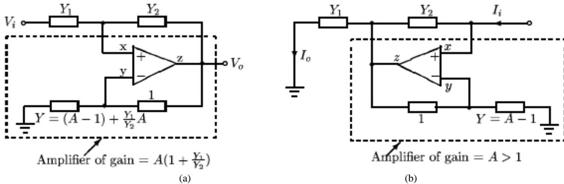
Fig. 12. (a) VM circuit and (b) CM circuit with active device having no input terminal at virtual ground.
