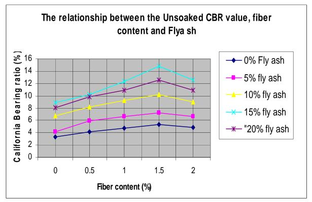
Clay soil. The results are shown in graph 1 and 2. For the 15% of fly ash and 1.5 % of the fiber maximum CBR is obtained.
