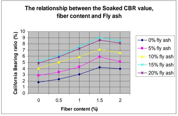
Graph-2, Variation of CBR for soaked condition with and without addition of fibers to the fly ash Soil
