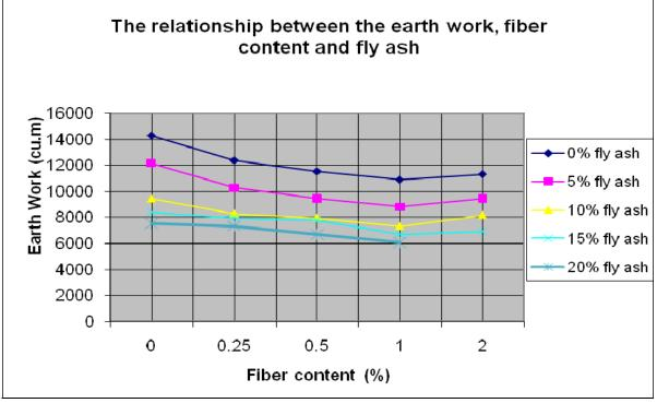
The relationship between the earth work, fiber content and fly ash for unsoaked condition is presented in the Graph 5.
