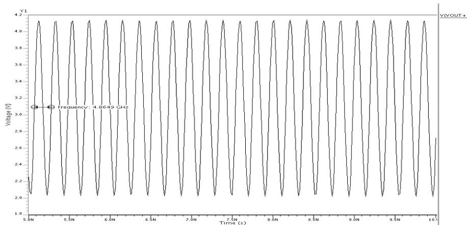
Fig. 7. Output waveform of proposed DCO at 0000H
