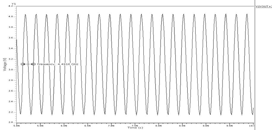
Fig. 6. Output waveform of conventional DCO at 0000H
