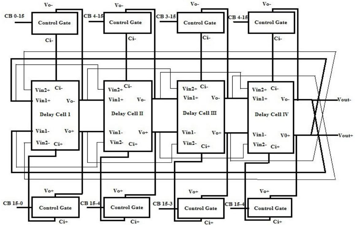
Fig. 3. DCO structure with dual delay paths scheme
