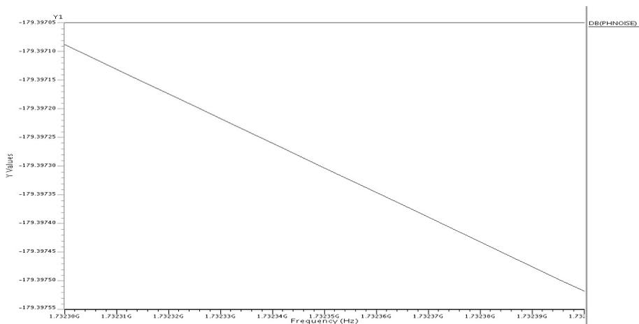
Fig. 9. Phase noise of DCO at FFFFH control word
