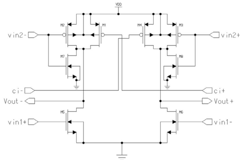
Fig. 4. The proposed four input differential delay latch cell
