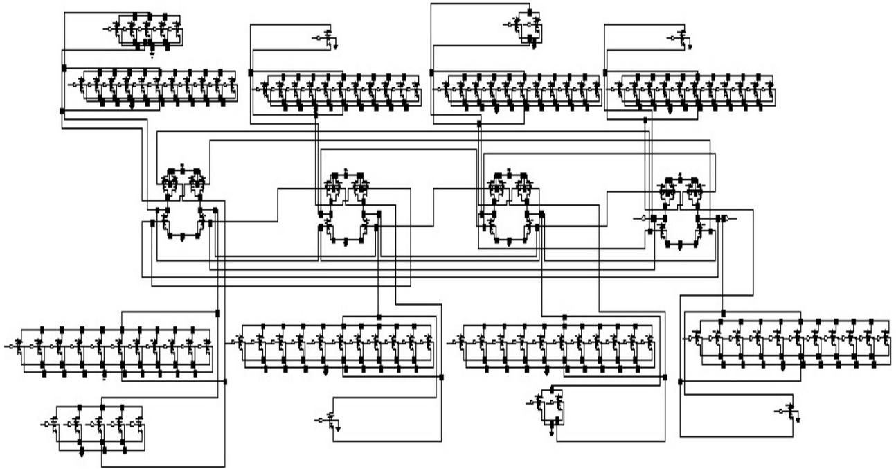
Fig. 3. A 16-bit digital controlled oscillator using a 4-stage proposed differential delay cell
