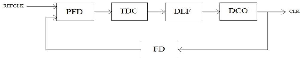
Fig. 1. Block diagram of ADPLL
