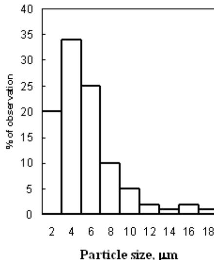
Fig.4 Size distribution of SiC after extrusion
