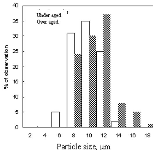
Fig.7 Size distribution of SiC present on the fractured surface of tensile tested specimen
