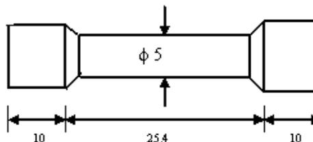
Fig.1 Tensile specimen tested. Dimensions are in mm.
