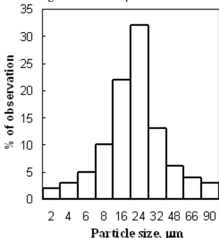
Fig.3 Size distribution of SiC prior to extrusion
