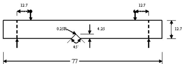
Fig.2 Notched bend bar tested. Dimensions are in mm.
