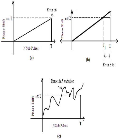
Fig. 2 Doppler phase shift on received bi-phase sequences (a) when phase shift is equal to  $\pm\pi/2$  (b) when phase shift is greater than  $\pm\pi/2$  (c) when additive noise is added along with Doppler phase shift.
