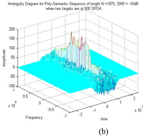
Fig. 10 shows the ambiguity diagram for poly-semantic sequences of length 1575, when two targets are at 500 SPDA (a) with no noise (b) with SNR of -10dB.
