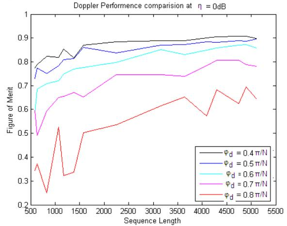
Fig. 6 Noise and Doppler performance of poly-semantic sequences at different Doppler phase shifts ( $\varphi_d$ ) and fixed  $\eta$  of 0 dB.
