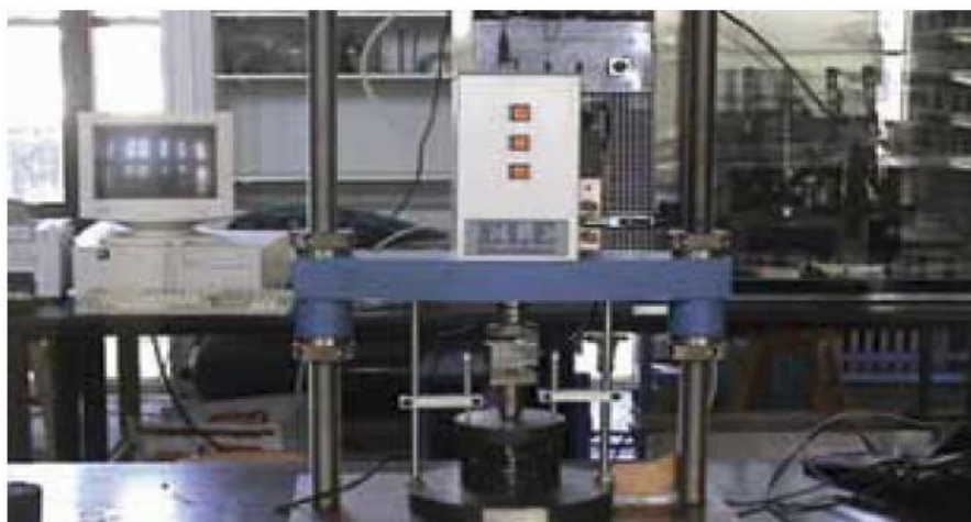
Figure 6: Specimen in the Static Creep Frame of a UTM.
