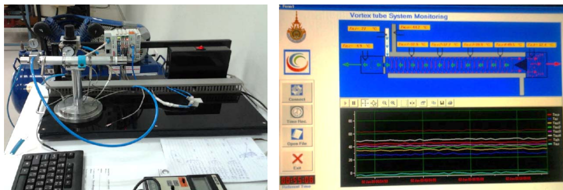
Fig.8 Experiment with the vortex tube data logger
