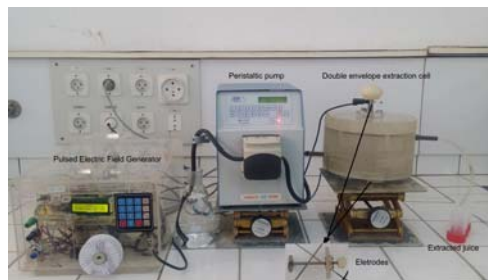
Fig. 1. : Experimental apparatus for PEF and thermal treatment
