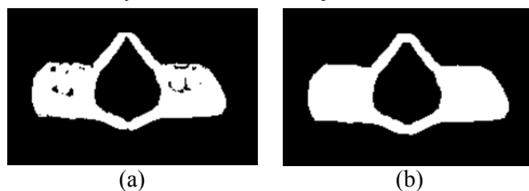
Fig. 4. (a) Binary image, (b) Binary image was resulted from the closing process
