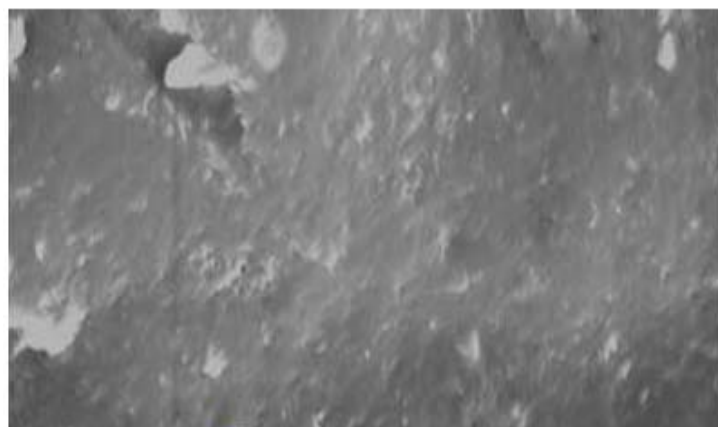
Fig. 7. SEM microstructure of 2.5 wt% nanoclay
