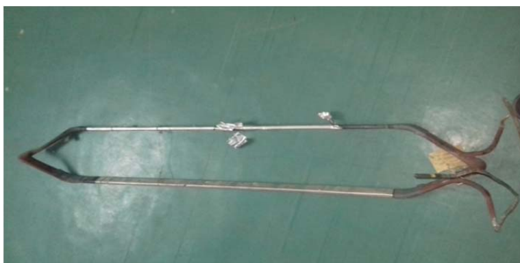
Fig.1. Snap shot of a 6.6 kV ten turn motor coil
